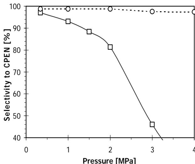
**Fig. 5.:** The influence of reaction pressure on selectivity of the hydrogenation at the CPD conversion 99.90%
