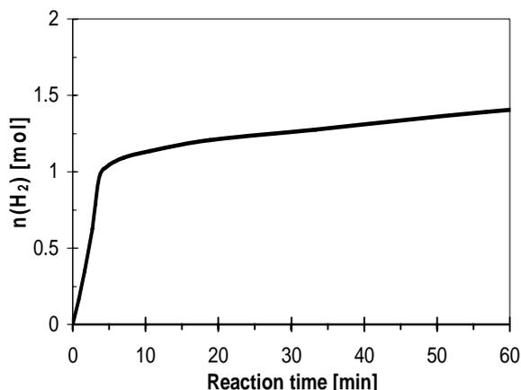
**Figure 1.** A typical course of the CPD hydrogenation on the selective Pd catalyst in powder form.  $n(H_2)$  – hydrogen consumption; 25°C, 2 MPa, 1.9 g 0.4% Pd/Al<sub>2</sub>O<sub>3</sub> (grains < 56 μm), 1 mol CPD as 10 wt.% solution in cyclohexane, batch slurry reactor of Set A.
