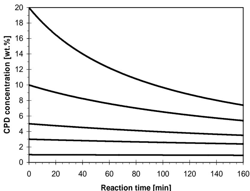
**Fig. 7.:** The drop in the CPD concentration in an inert solvent (cyclohexane) due to the spontaneous thermal dimerization of CPD at 25°C depending on the initial CPD concentration.
