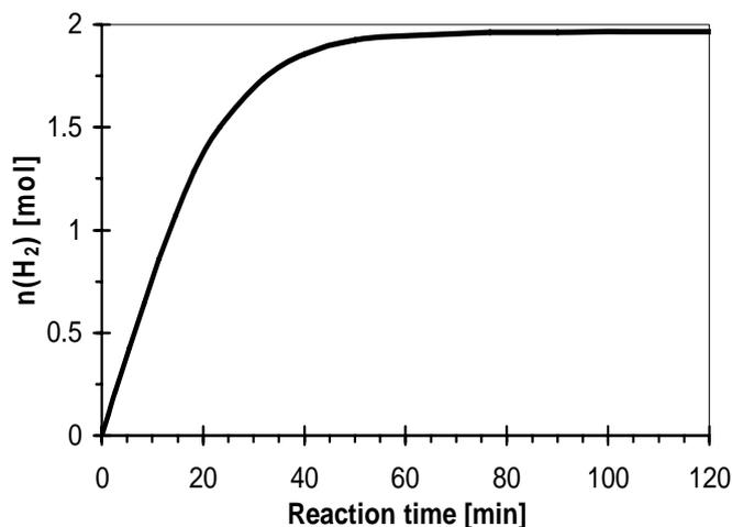
**Figure 2.** A typical course of the CPD hydrogenation on the high selectivity Pd catalyst in pellet form
