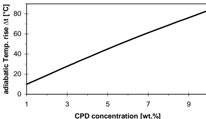
**Fig. 4.:** Dependence of the value of adiabatic temperature rise (in the liquid phase CPD hydrogenation) on the substrate concentration in the starting raw material. Initial material: CPD solution in cyclohexane, Values of adiabatic temperature rise in the moment when CPD reacted off for the hydrogenation with selectivity  $S_{CPEN}=80\%$ . Calculated from literature tabled thermo-dynamic data.
