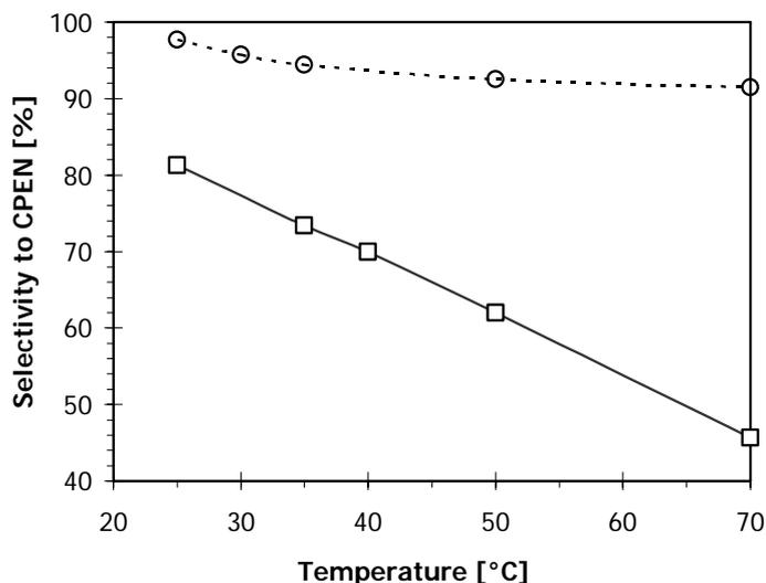
**Fig. 6.:** Effects of reaction temperature on selectivity of the hydrogenation at the CPD conversion 99.90%
