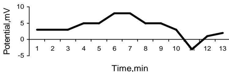
Figure 3. The dependence of the polarization potential from the time using manual injection
