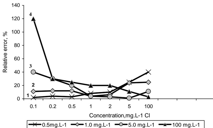
Figure 5. The relative error of the measurements in dependence of the calibration standard used
