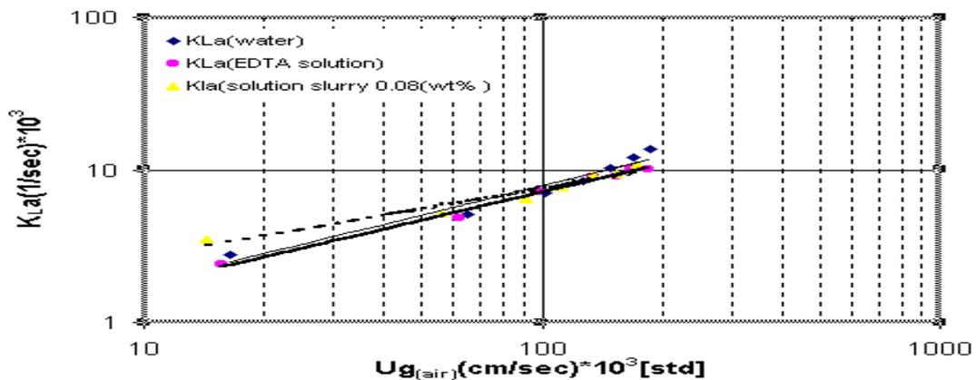
Figure 6. MTC vs. riser superficial gas velocity. Comparison of the oxygen MTC in water, EDTA solution (500ppm) and EDTA slurry solution 0.08(wt%)
