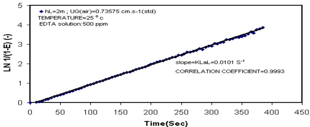
Figure 3. A typical  $1/(1-E)$  vs. time
