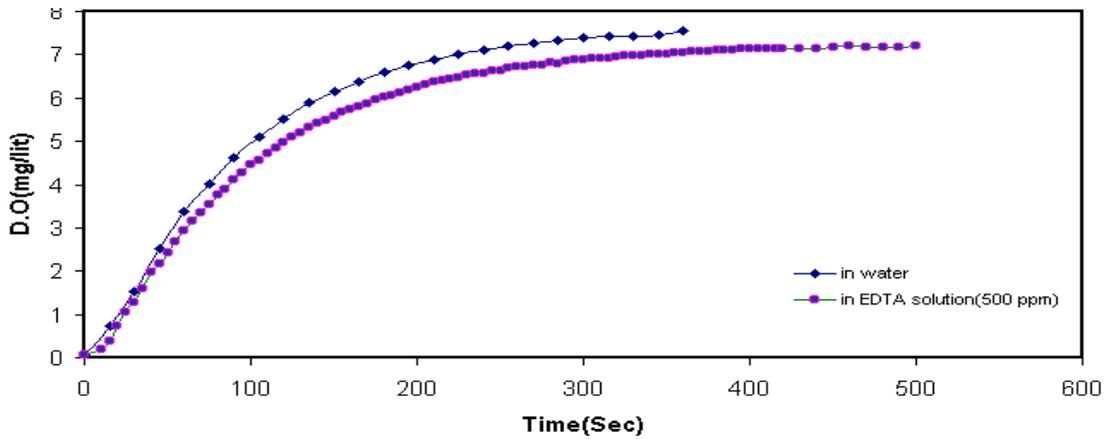
Figure 4. Effect Of Liquid Type on Dissolved Oxygen for EDTA solution
