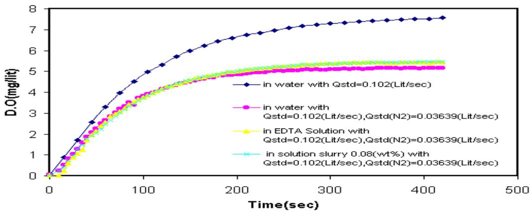
Figure 5. Effect of Nitrogen on Dissolved Oxygen for water, EDTA and slurry solution
