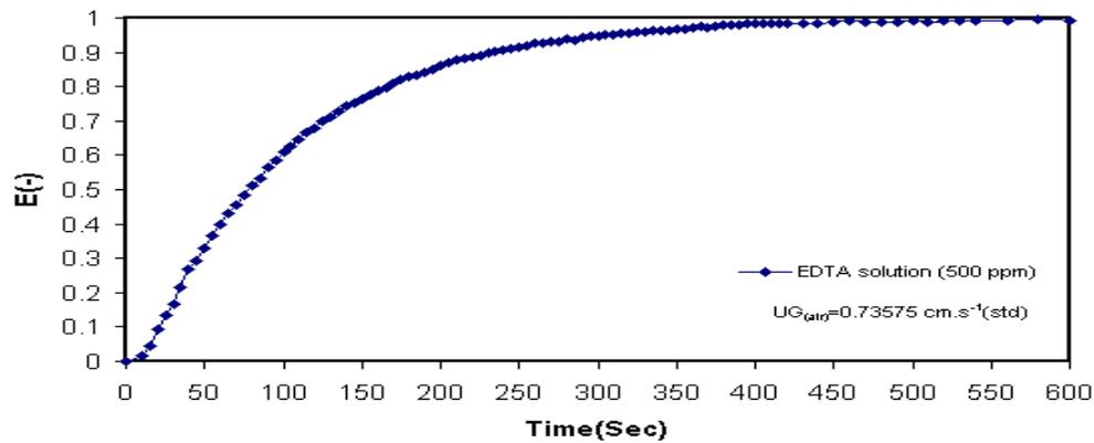
Figure 2. A typical E vs time profile for Air-EDTA
