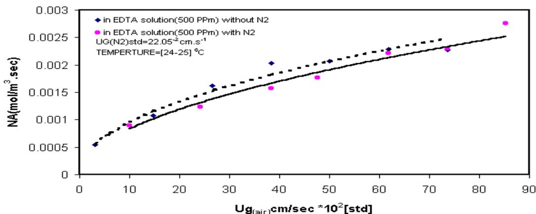
Figure 8. Effect of Nitrogen on Mass Transfer Flux; NA
