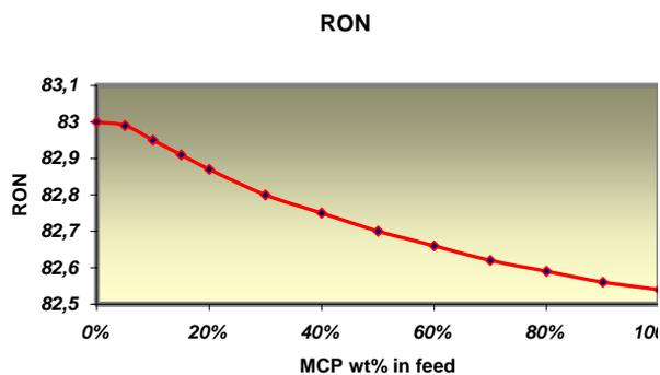
Fig. 2- Effect of increase of MCP weight percentage on RON of the final product
