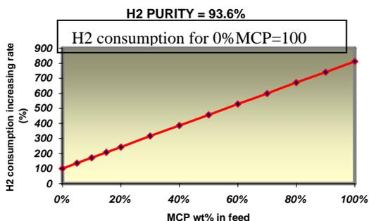
Fig. 3- Effect of increase of MCP weight percentage on make up hydrogen
