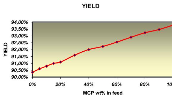
Fig. 3- Effect of increase of MCP weight percentage on process yield
