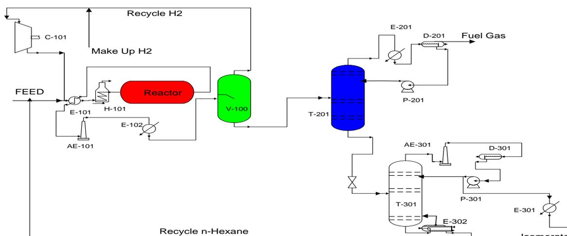
Fig. 1 - Block diagram of isomerization process for the 13 case studies
