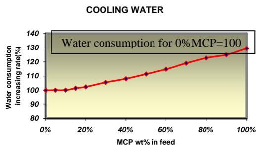
Fig. 5- Effect of increase of MCP weight percentage on cooling water consumption
