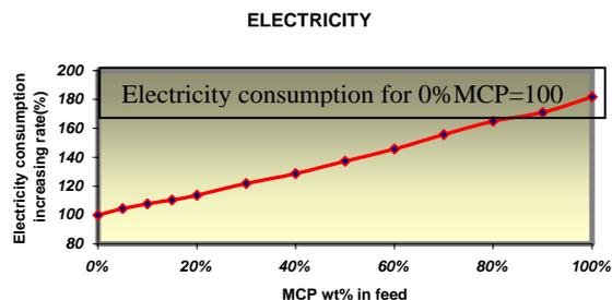
Fig. 6- Effect of increase of MCP weight percentage on electricity consumption
