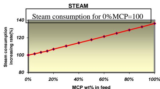
Fig. 4- Effect of increase of MCP weight percentage on steam consumption
