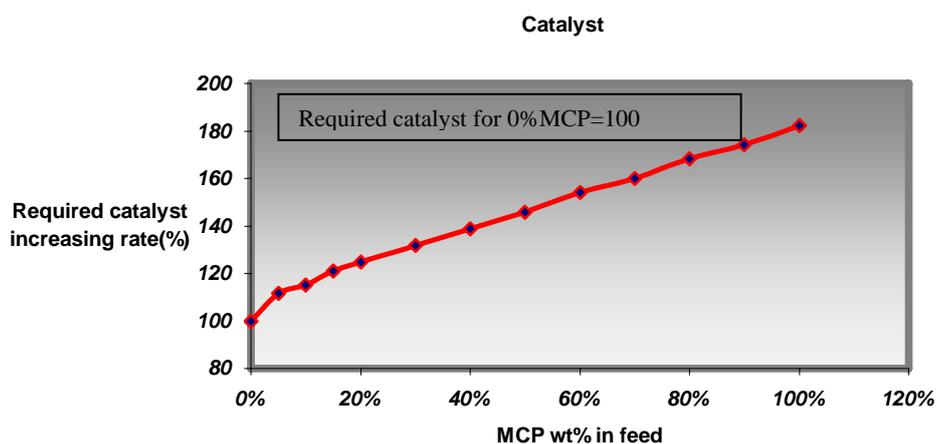
Fig. 8- Effect of increase of MCP weight percentage on catalyst consumption
