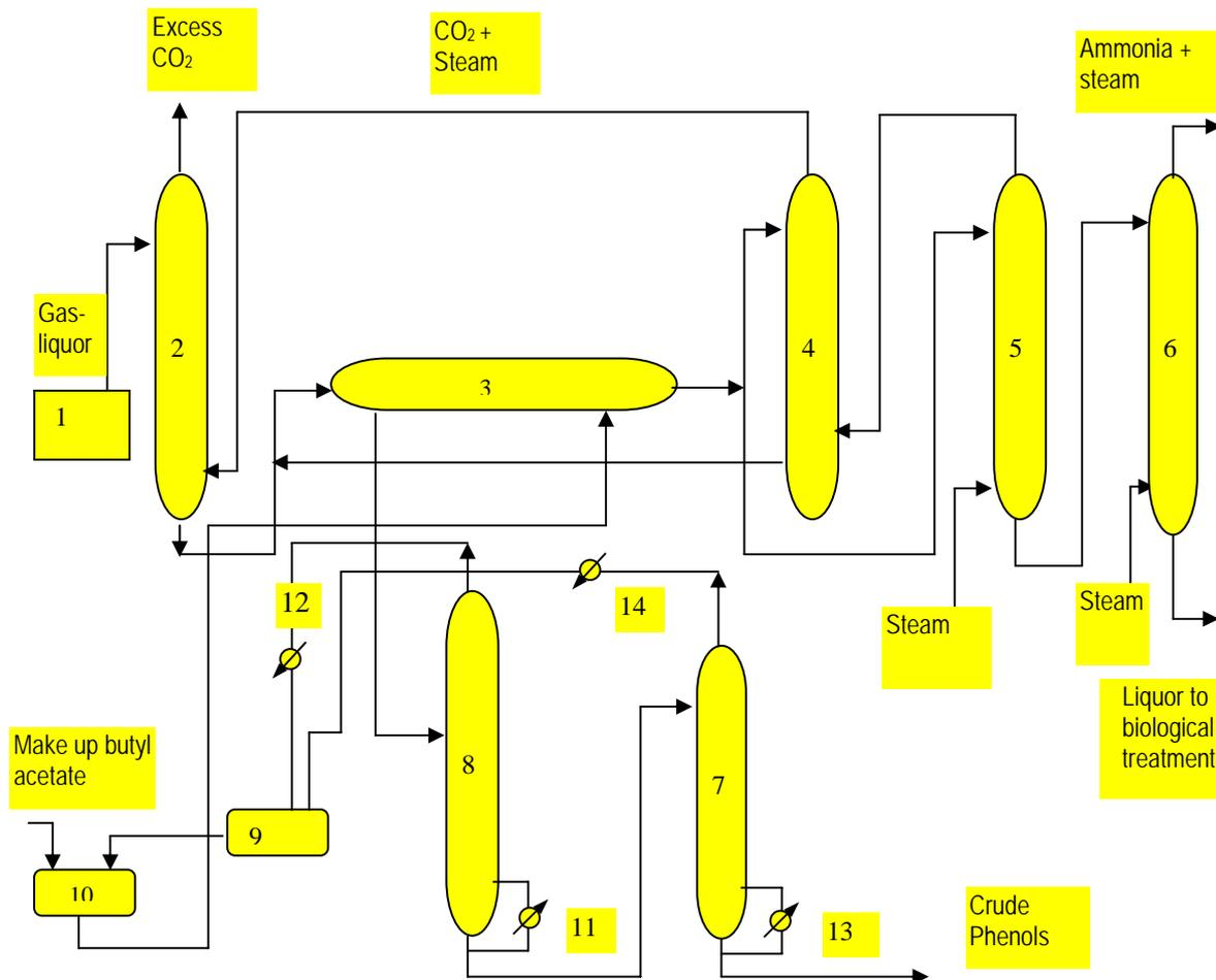
Figure 1. Phenol recovery plant. 1-Tar-oil separation; 2- Saturation tower; 3- Phenol extractor; 4- Butyl-acetate recovery tower; 5- Butyl-acetate stripping tower; 6- Ammonia stripping tower; 7- Atmospheric distillation tower; 8- Vacuum distillation tower; 9- Separator drum; 10- Butyl-acetate circulating drum
