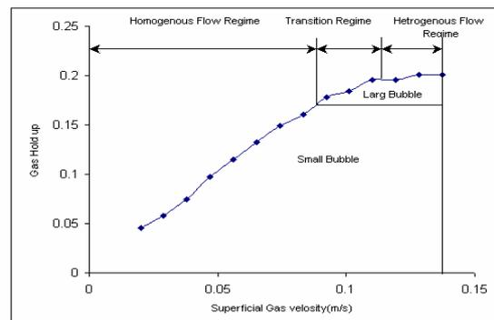
Fig 2 Effect of superficial gas velocity on gas hold up in air-water system
