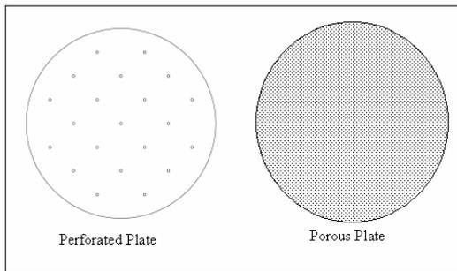
Fig 5 Two sparger types are used in the experimental set up
