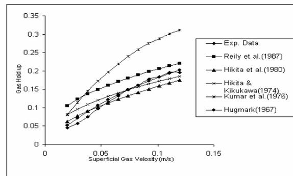
Fig 4 Comparison between correlations and experimental data
