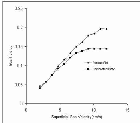
Fig 7 Effect of sparger type on gas hold up
