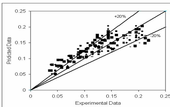
Fig 3 Comparison between predicted value and experimental data of gas hold-up
