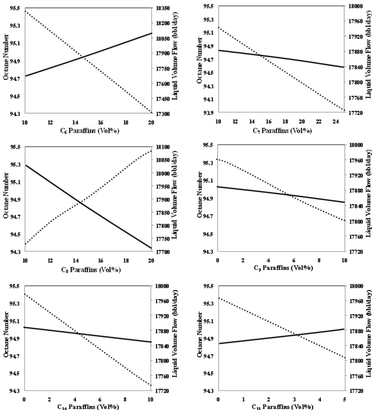
Fig. 5 The effects of paraffins feedstock composition on final product octane number, (solid line) & liquid volume flow (dotted line)
