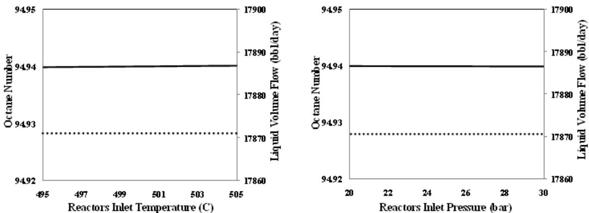
Figure2. The effects of reactor’s inlet temperature and pressure on final product octane number (solid line) & liquid volume flow (dotted line)
