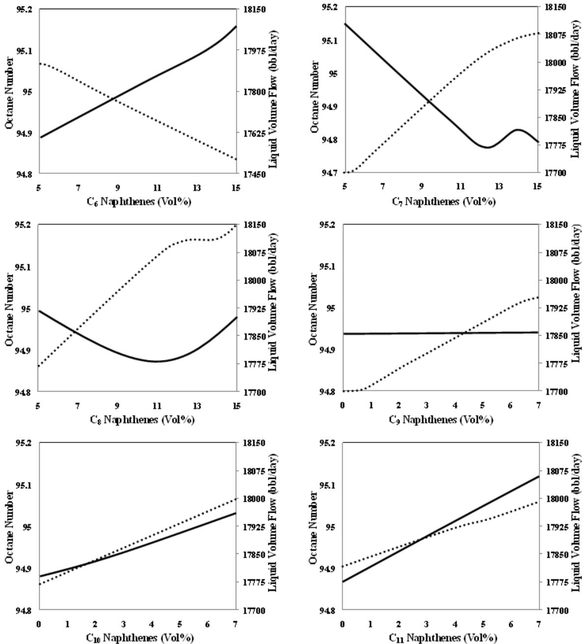
Fig. 4 The effects of naphthenes feedstock composition on final product octane number, (solid line) & liquid volume flow (dotted line).
