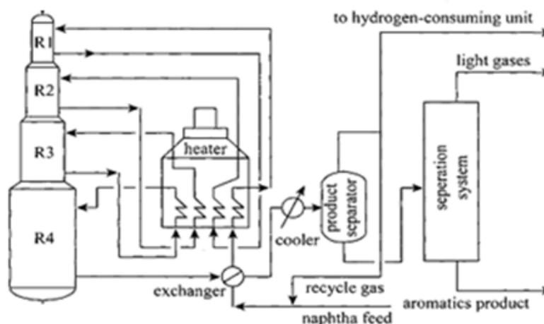
Fig. 1 Catalytic reforming flowsheet (semi-regenerative)
