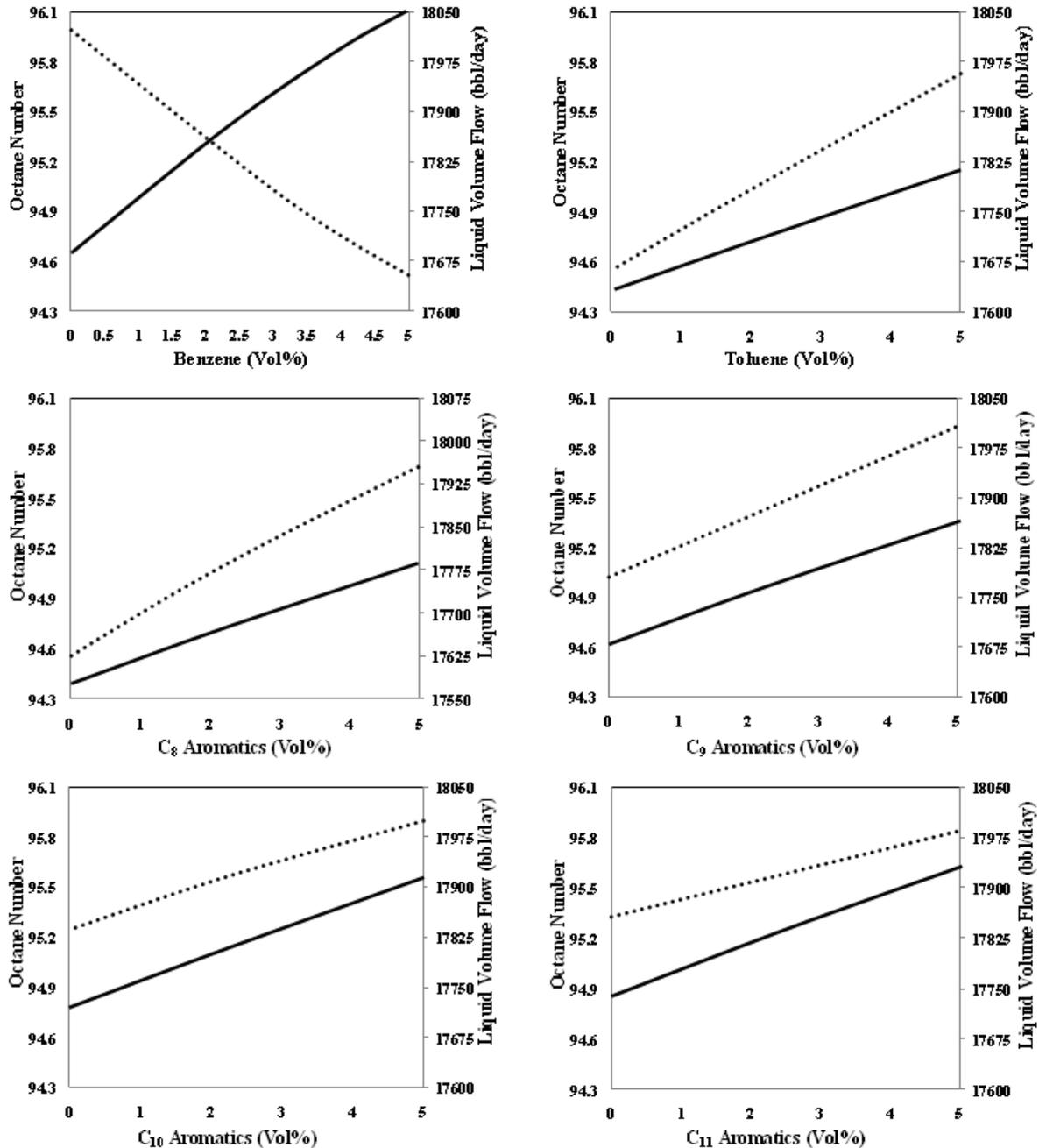
Fig. 3. The effects of aromatics feedstock composition on final product octane number, (solid line) & liquid volume flow (dotted line).
