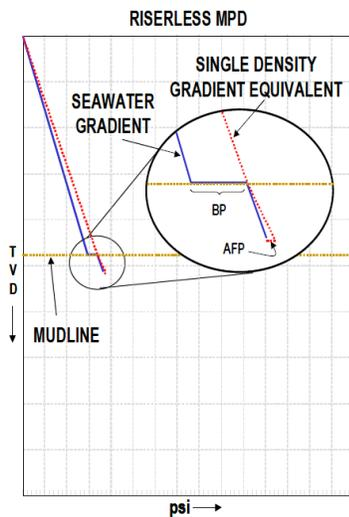
Fig. 9. Pressure profile for drilling dual gradient without a riser [16]
