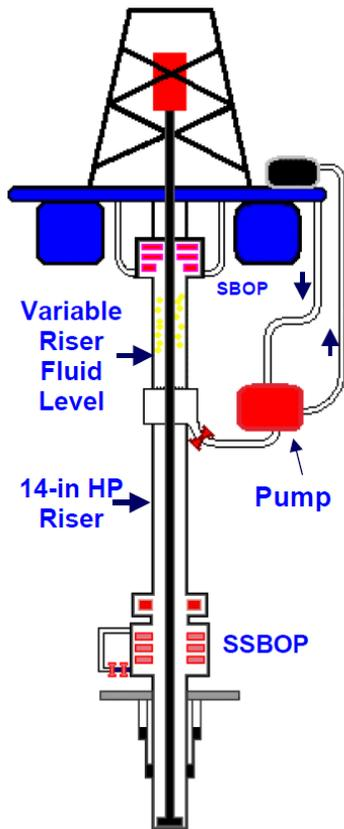
Fig. 7. Controlled mud cap setup [9]
