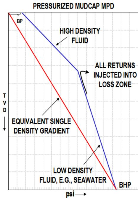
Fig. 5. Pressure-gradient profile for pressurized mud cap drilling method [16]
