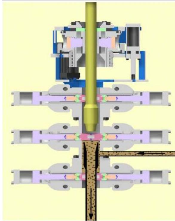
Fig. 4. Coupler device used in the continuous circulation system [13]
