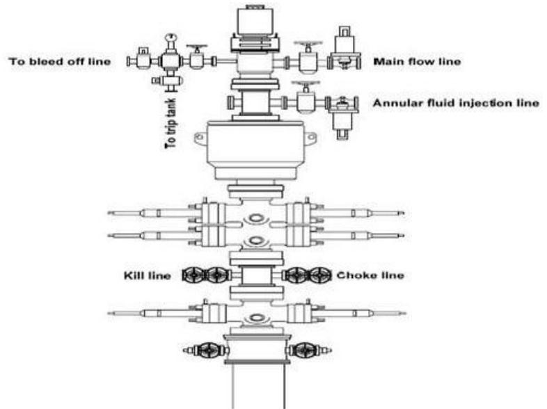
Fig. 6. Rig up for Pressurized Mud Cap Drilling Operations [12]
