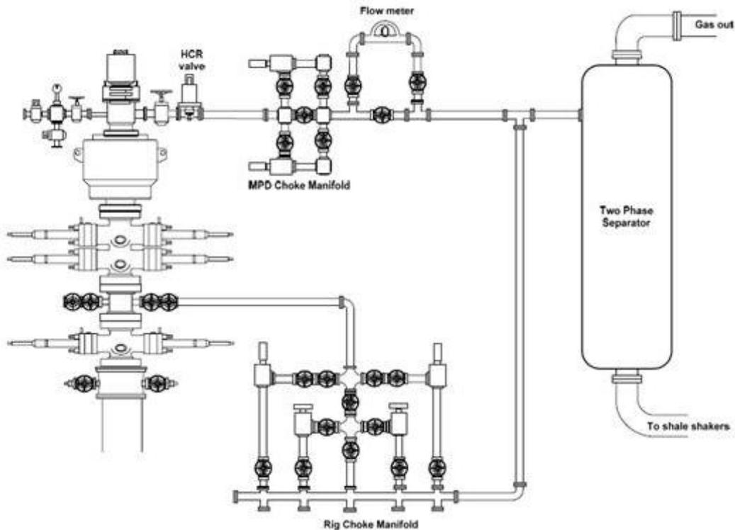
Fig. 3. Rig up for CBHP applications. [12]
