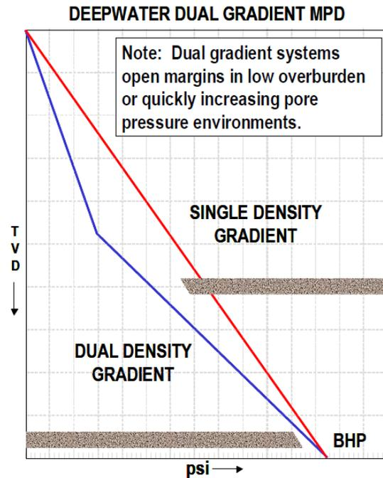
Fig. 8. Dual-gradient drilling pressure gradient profile [16]
