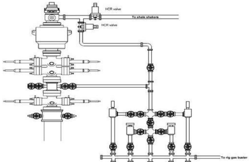
Fig. 10. MPD rig up for Return Flow Control [12]
