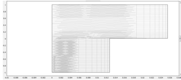
Fig. 5. Boundary layer grid for finite element analysis
