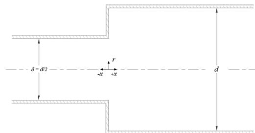
Fig. 1. The computational domain and geometry specifications
