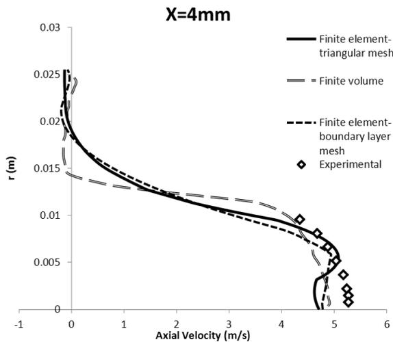
Fig. 6. Variation in the axial velocity at X=4mm
