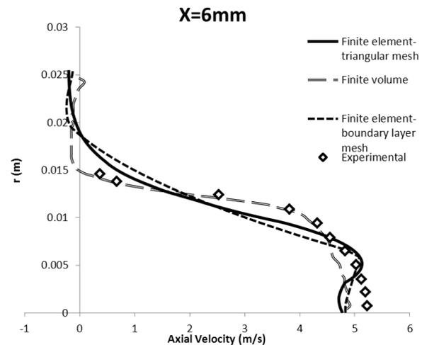
Fig. 7. Variation in the axial velocity at X=6mm
