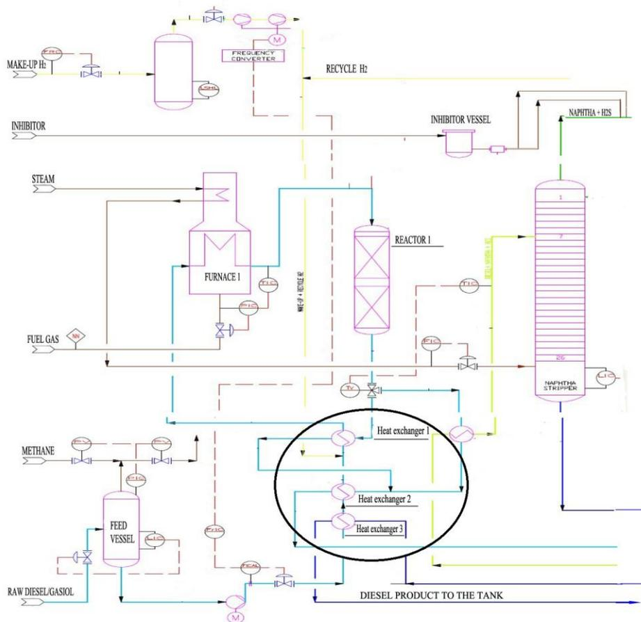
Fig. 1 Scheme of HDS plant in Insa oil refinery
