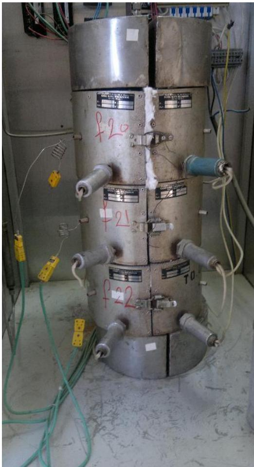
Figure 1 FTS fixed-bed reactor
