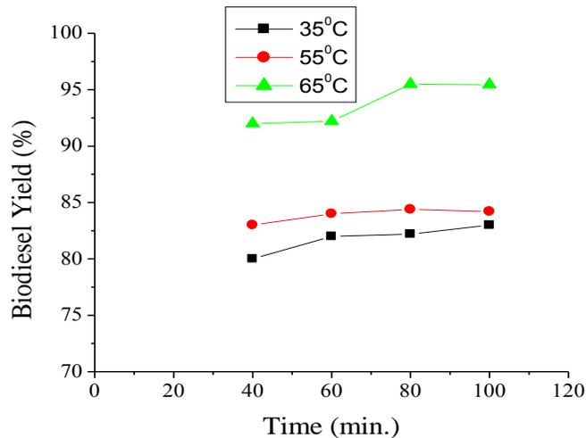
Fig. 3 Effect of temperature on transesterification
