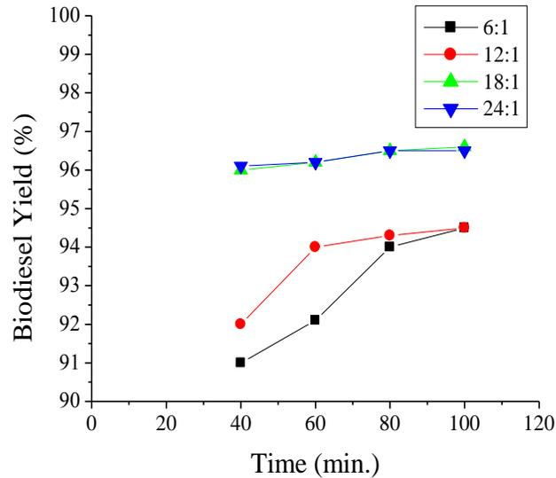
Fig. 2 Effect of ethanol-oil ratio on transesterification reaction
