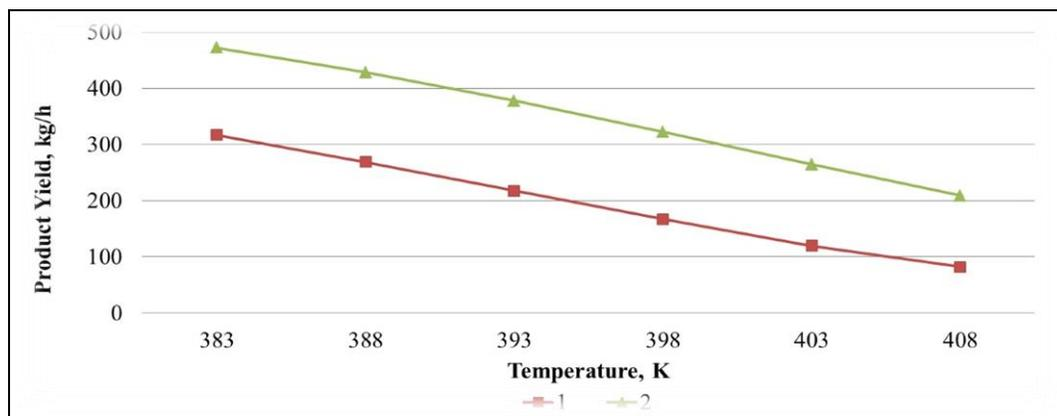
Figure 2. Dependence of diethylbenzene on temperature for two various feed compositions
