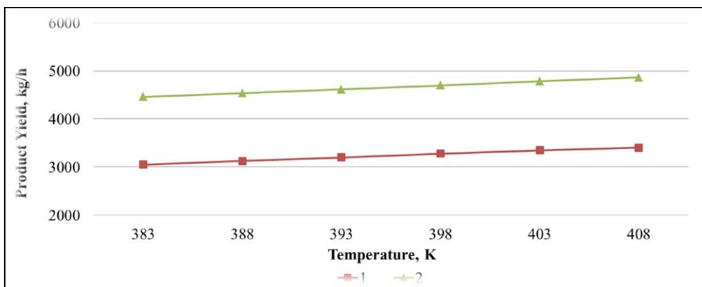
Figure 1. Dependence of ethylbenzene yield on temperature for two various feed compositions
