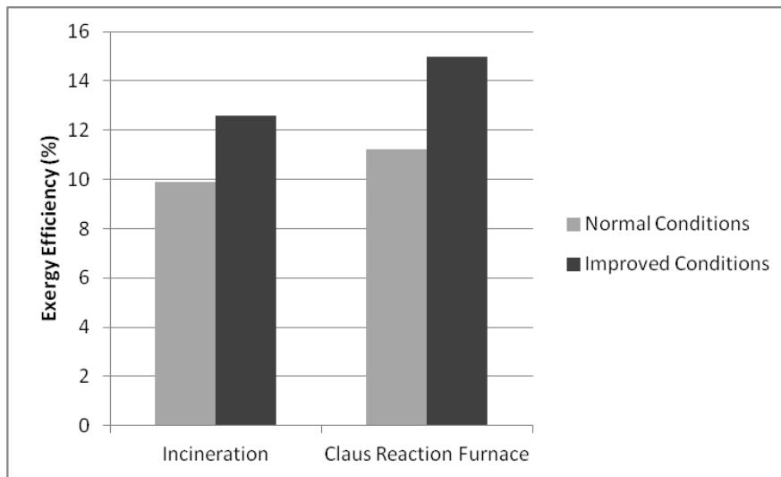
Fig.3 Enhancement of exergy efficiency by improving the conditions
