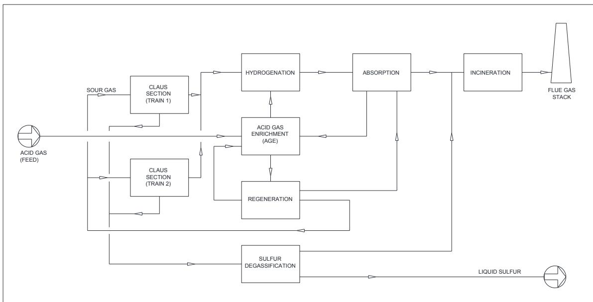
Fig. 1 Block Flow Diagram of Sulfur Recovery Unit
