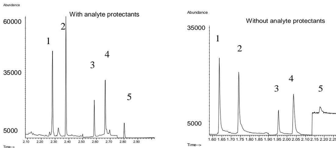
Fig. 4. SIM chromatograms of explosives with and without analyte protectants, concentration 0.1 ng/ $\mu$ l, injection volume 2  $\mu$ l; other experimental conditions - in experimental part; 1 – 2,6 DNT, 2 – 2,4 DNT, 3 – TNT, 4 – pentrite, 5 – RDX.
