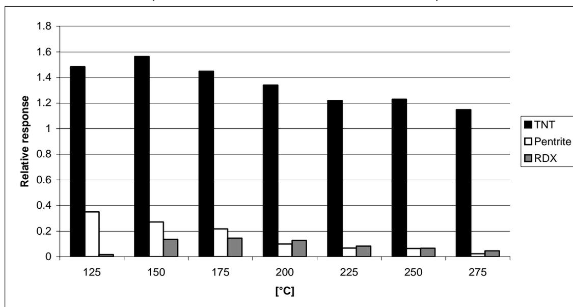
Fig. 1. Average relative response ( $n=3$ ), calculated to 2,6 DNT, for problematic compounds in the dependence on temperatures of PTV in splitless mode, concentration 10 ng/ $\mu l$ , injected volume 0.5  $\mu l$ .
