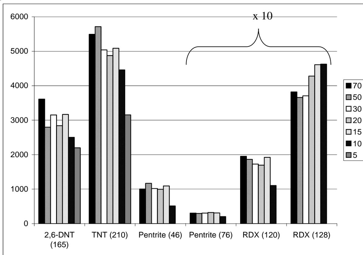
Fig. 3. Dependence of signal to noise ratios of explosives for EI electron energies, injected volume 1  $\mu$ l, concentration 10 ng/ $\mu$ l.
