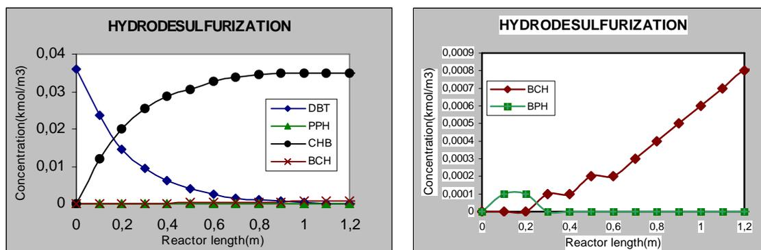
Figure 9. Concentration Profiles along Reactor Length. The reactor conditions are presented in Table 2.
