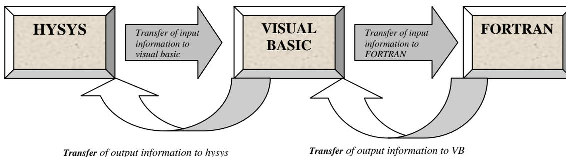
Fig. 7. Information flow diagram of the simulation software
