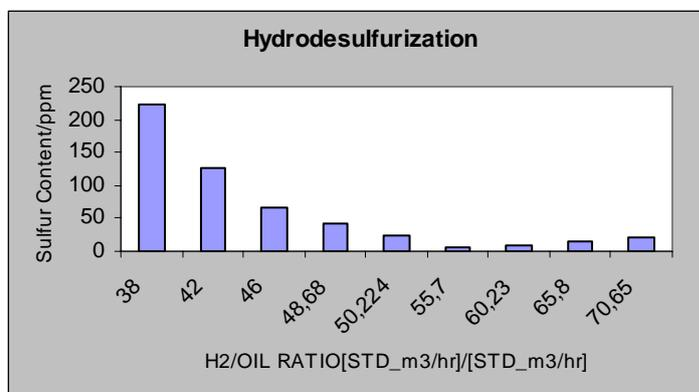
Figure 12. Effect of  $H_2$ /oil ratio on sulfur concentration in the treated gas oil. The input characteristics of the simulation are presented in table 3
