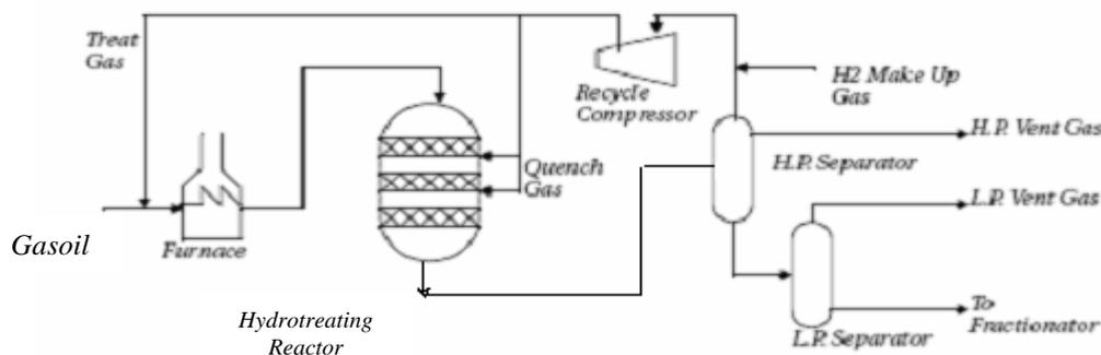
Fig.6. Schematics of hydrodesulfurization process
