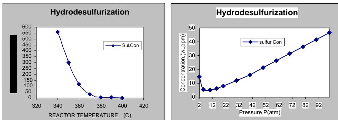
Figure 10. Effect of reactor temperature on sulfur concentration in the treated gas oil. The input characteristics of the simulation are presented in table 3.
