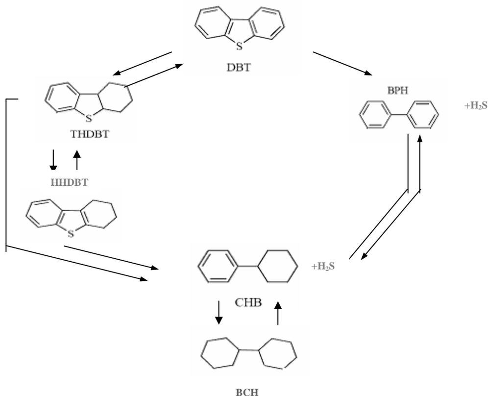
Fig 2. Reactions network for HDS of DBT <sup>[15]</sup>
