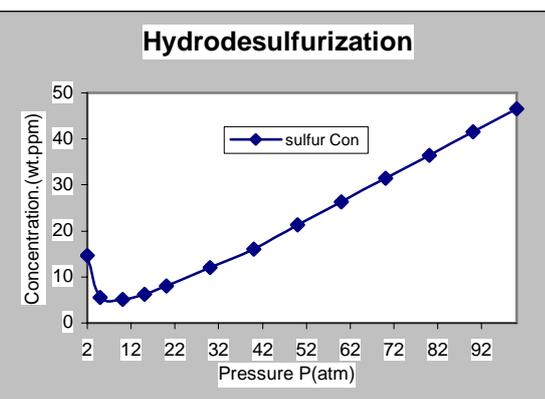
Figure 11. Effects of reactor pressure on sulfur Concentration in the treated gas oil. The input characteristics of the simulation are presented in table 3
