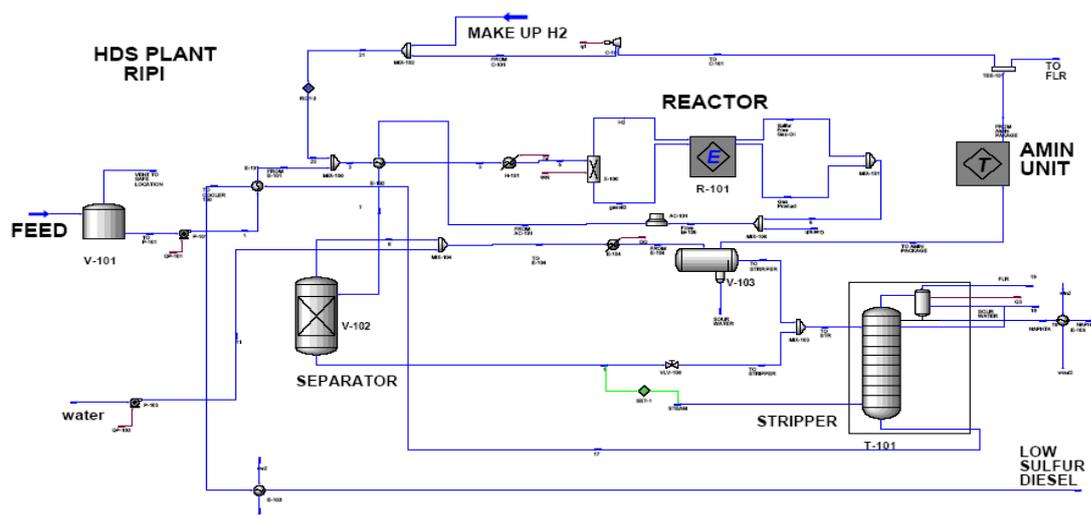
Fig. 8. PFD of Process simulated by HYSYS. The reactor model results are implemented interactively to the simulation environment
