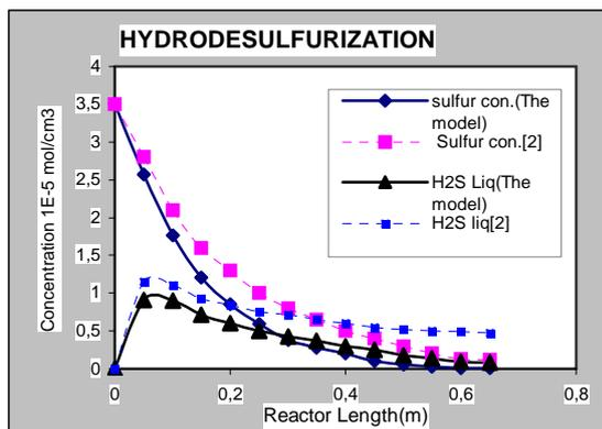
Fig.4. Sulfur & H<sub>2</sub>S concentration profile
