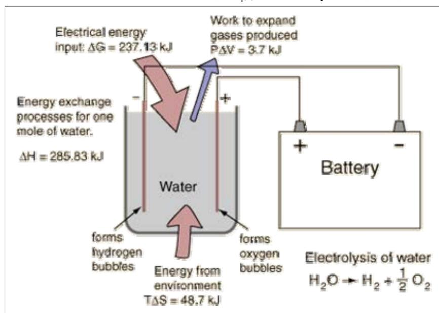
Figure 1: Electrolysis scheme
