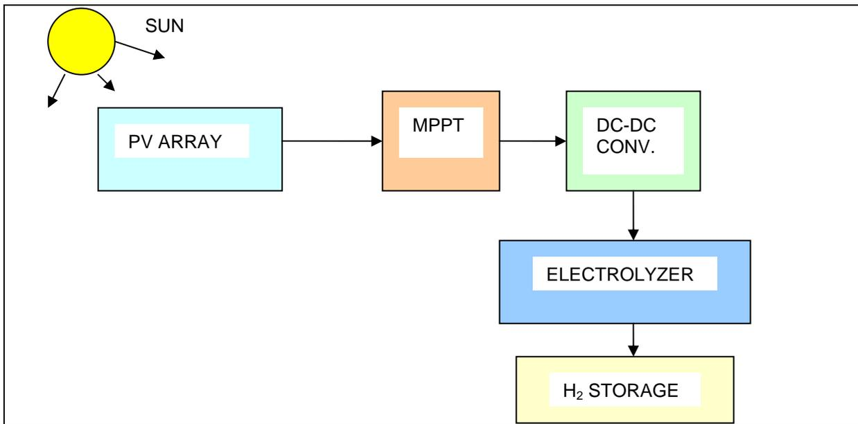
Figure 2 : Schematic of PV – hydrogen production system [5]
