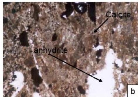
Fig: 5b. Polished thin section showing anhydrite as microgranular and prismatic-aligned fibre (x 40)
