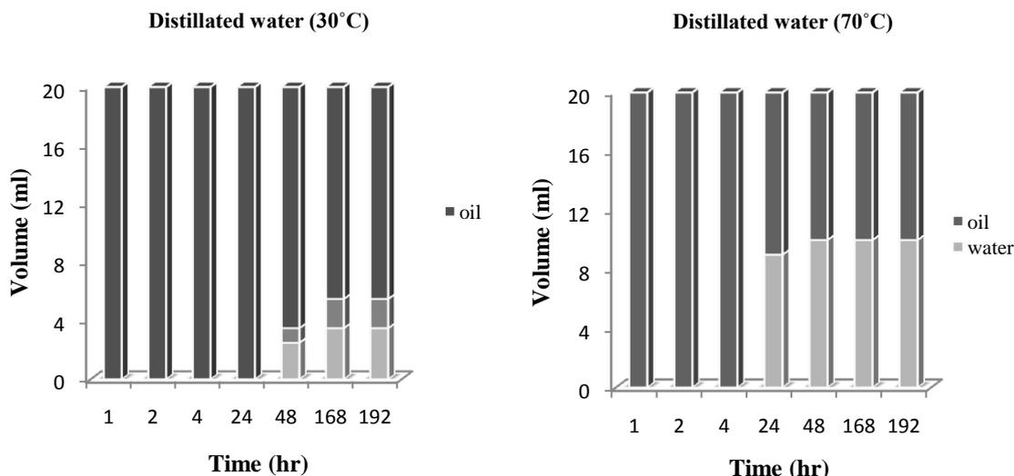
Figure 1. Effect of temperature on emulsion stability with distilled water
