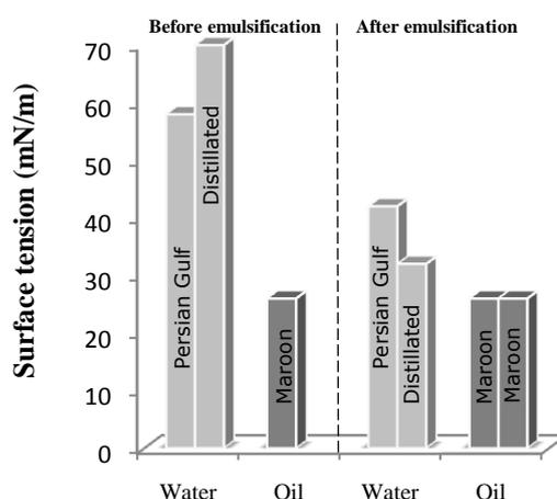
Figure 6. Surface tension of individual w/o phases before and after emulsification
