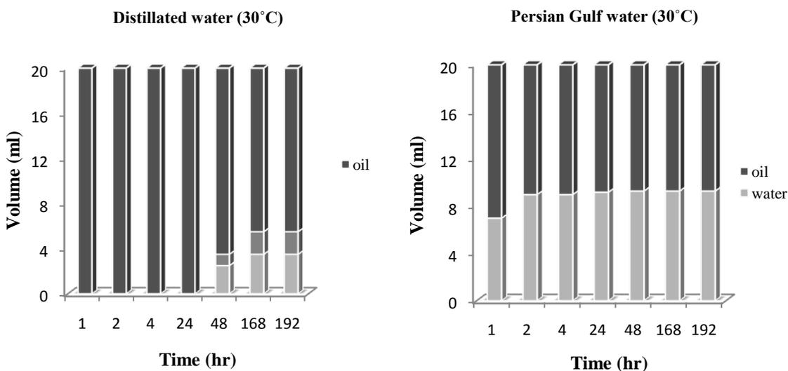
Figure 2. Effect of water quality (ionic strength) on emulsion stability
