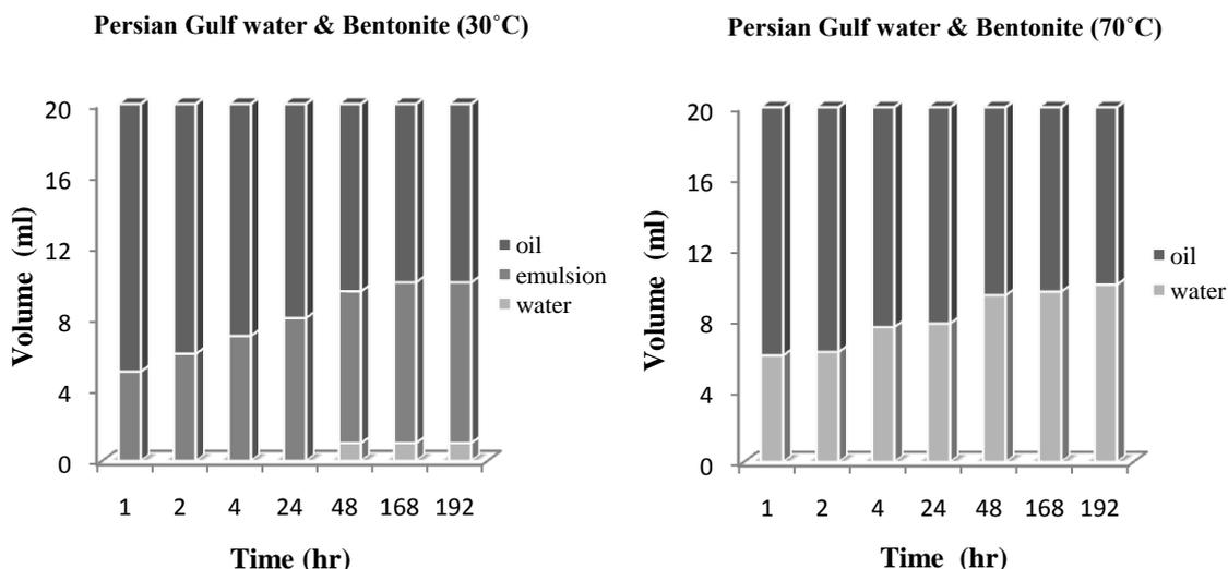
Figure 4. Effect of bentonite on emulsion stability with Persian Gulf water
