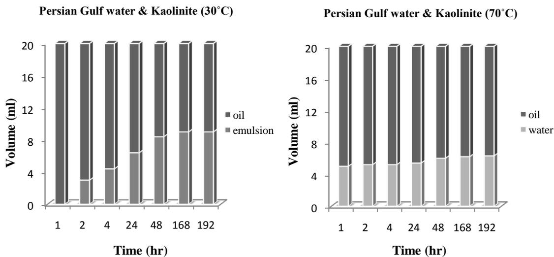
Figure 5. Effect of kaolinite on emulsion stability with Persian Gulf water
