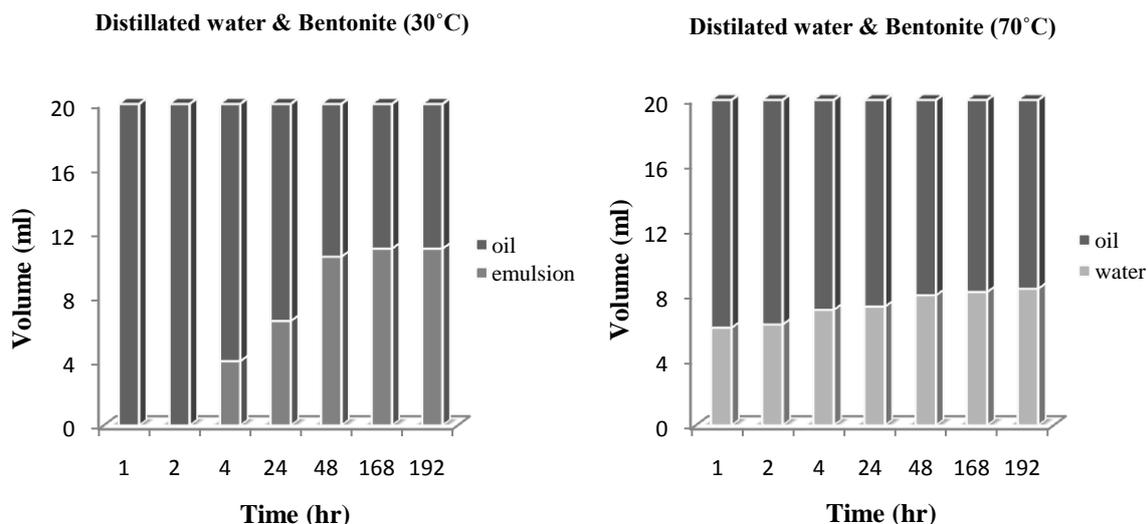
Figure 3. Effect of bentonite on emulsion stability with distilled water
