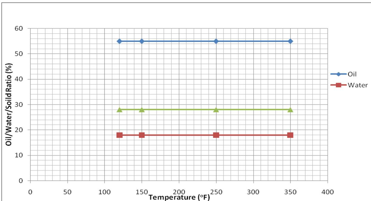
Fig. 9 Effect of aging on oil/water/solid ratio of Versaclean mud
