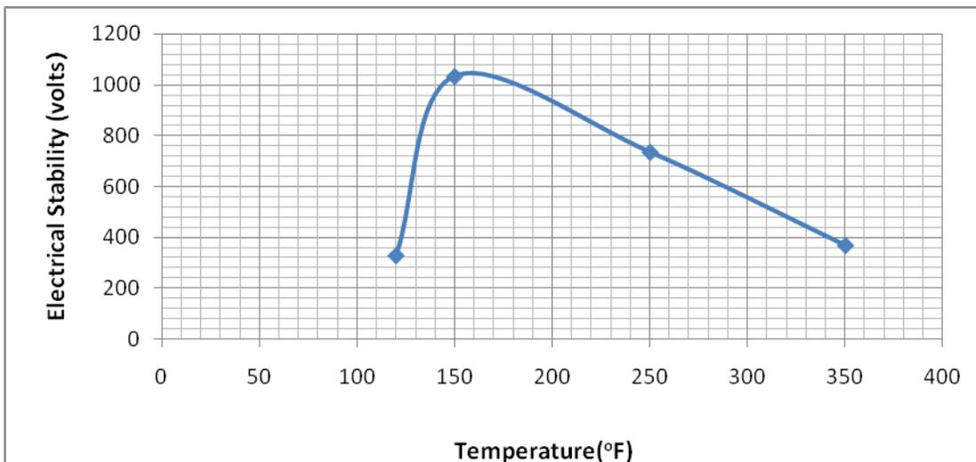
Fig. 6 Effect of aging on electrical stability of Versaclean mud
