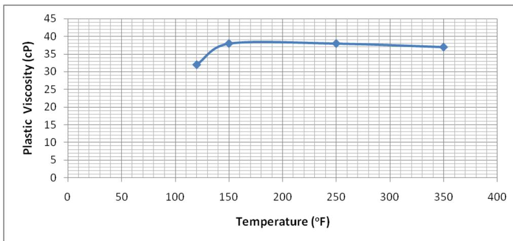
Fig.3 Effect of aging on plastic viscosity of Versaclean mud
