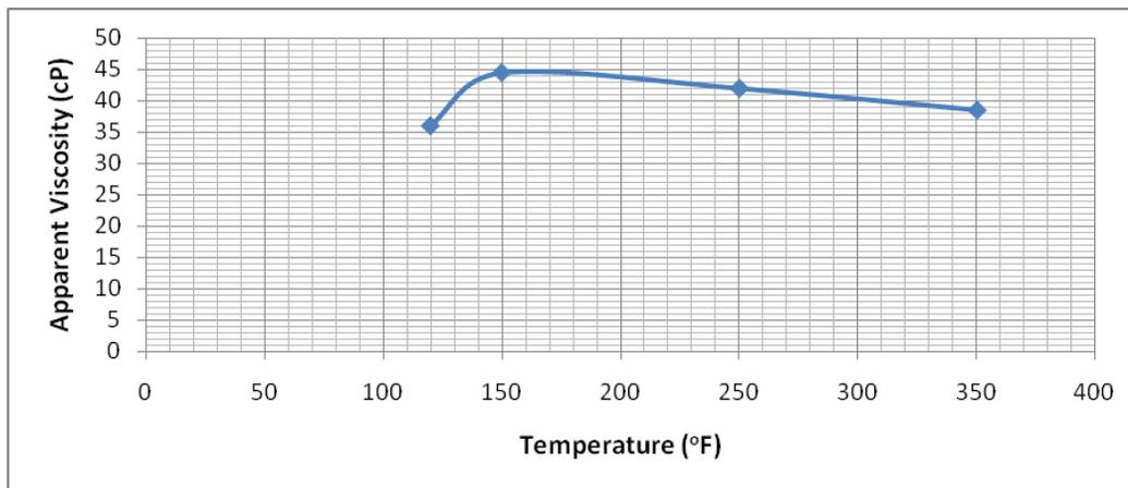
Fig.2 Effect of aging on apparent viscosity of Versaclean mud
