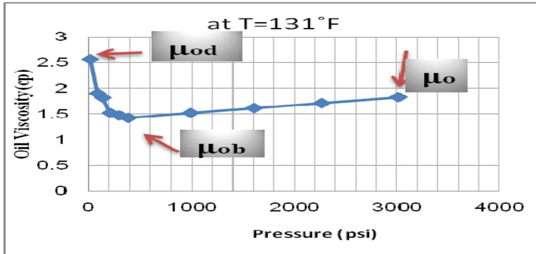
Statistical experimental data are shown in table 1. At pressures above bubble point pressure, oil is at single-phase state, while its solution gas-oil is constant and it seems that pressure will be the most effective in oil viscosity.
