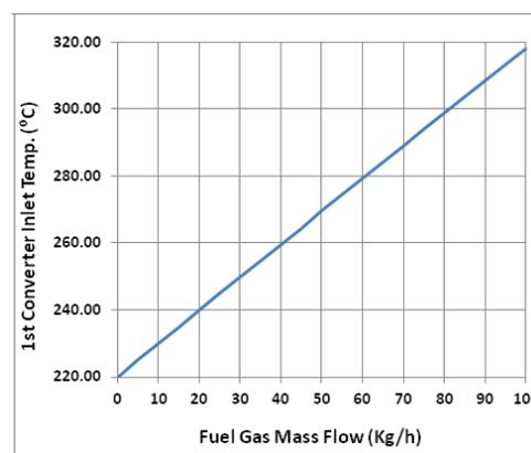
Fig. 4. The changes in temperature of first converter inlet stream vs. mass flow rate of fuel gas inserting into the inline burner
