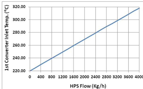
Figure 2. The changes of HPS mass flow vs. the temperature of first converter inlet stream
