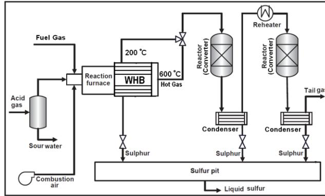
Figure1. A schematic shape of a modified two-stage Claus process with acid gas and air preheating and hot gas configurations
