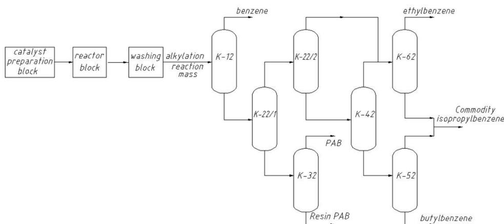
Figure 1. Simplified flow diagram of IBP production on chloroaluminum catalyst
