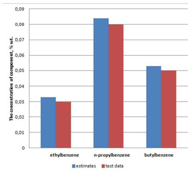
Figure 2. Comparative analysis of calculated and monitoring data on the yield of commercial IPB (in 2015 year)
