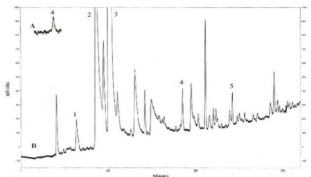
Figure 2. **A:** Peak of benzene at 0.05 ng/microcolumn, **B:** Chromatogram of exhaled breath sample (100 ml), peaks: 1:methanol, 2:ethanol, 3:acetone, 4:benzene ( $4,7 \mu\text{g}/\text{m}^3$ ), 5:toluene.
