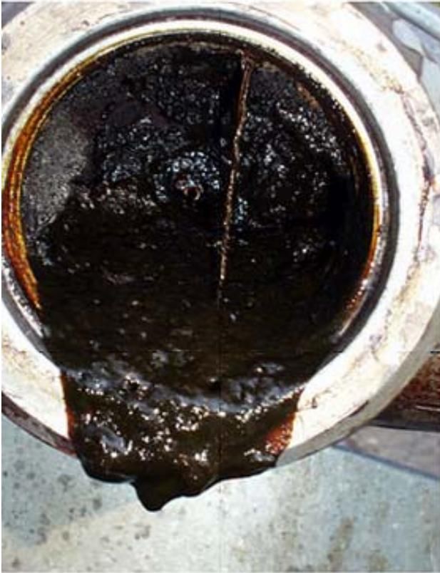
Picture 3 Transport duct of crude oil before the application of the means
