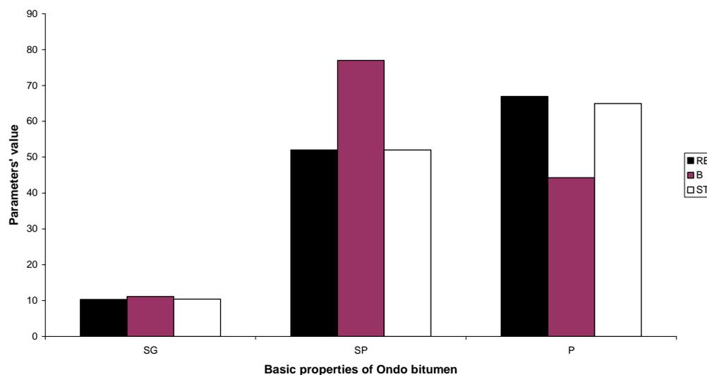
Fig. 1: Comparison of the specific gravity (SGX10), softening point (SP) and penetration (P) of Ondo bitumen as-received (B) and refined (RB) with standard (ST)
