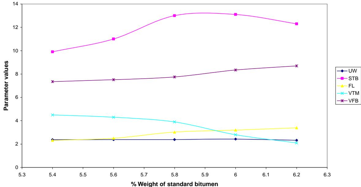
Fig.2: Variation of unit weight (UW), stability (STB), flow (FL), % voids in total mix (VTM) and % total voids filled with bitumen (X0.1 VFB) in HMAC with % bitumen
