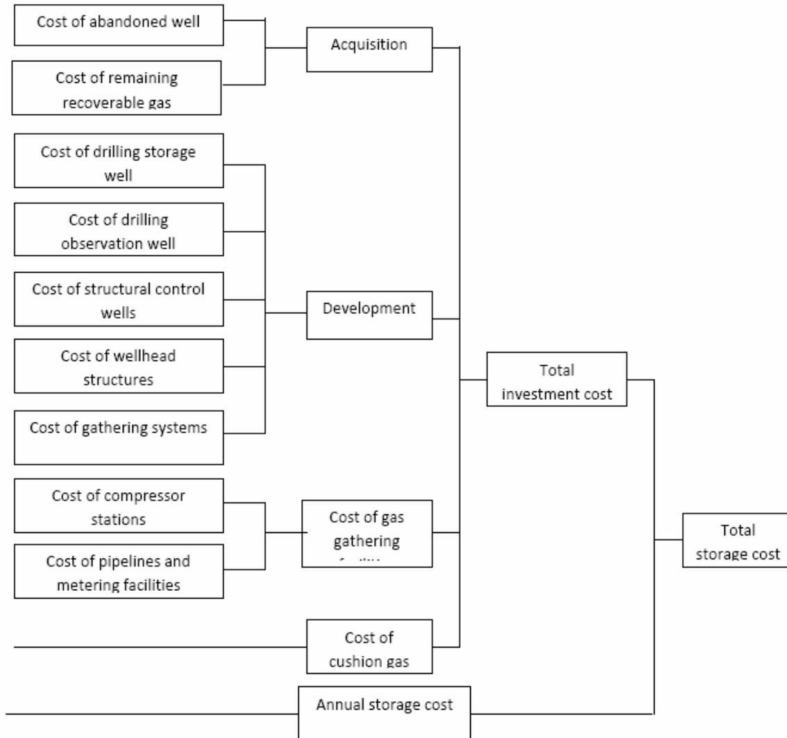
Fig 1 Economic flow chart for natural gas storage in depleted reservoir
