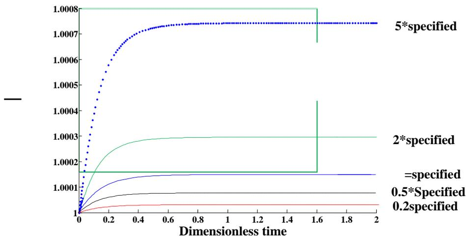
Fig. 8. Variation of pellet temperature with time
