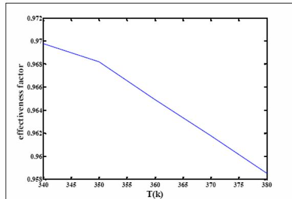
Fig. 4 Variation of effectiveness factor with surface temperature
