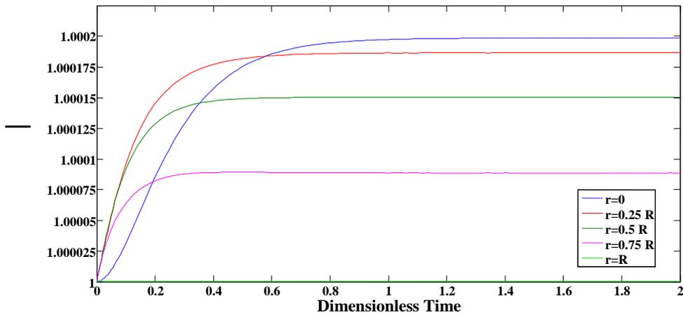
Fig. 6 Temperature profile for catalyst pellet in dynamic mode
