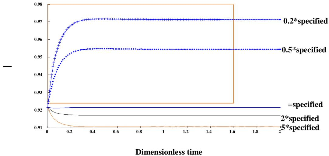
Fig. 7. Variation of pellet concentration with time
