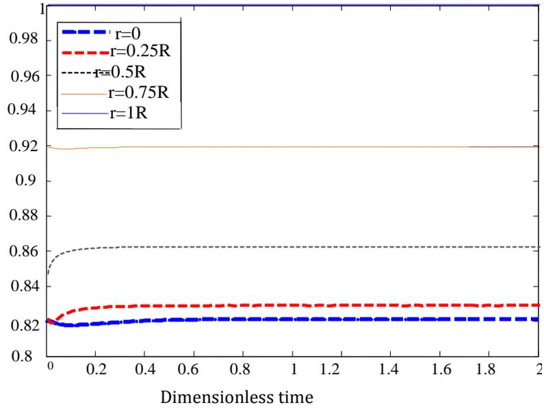
Fig.5 Concentration profile for catalyst pellet in dynamic mode
