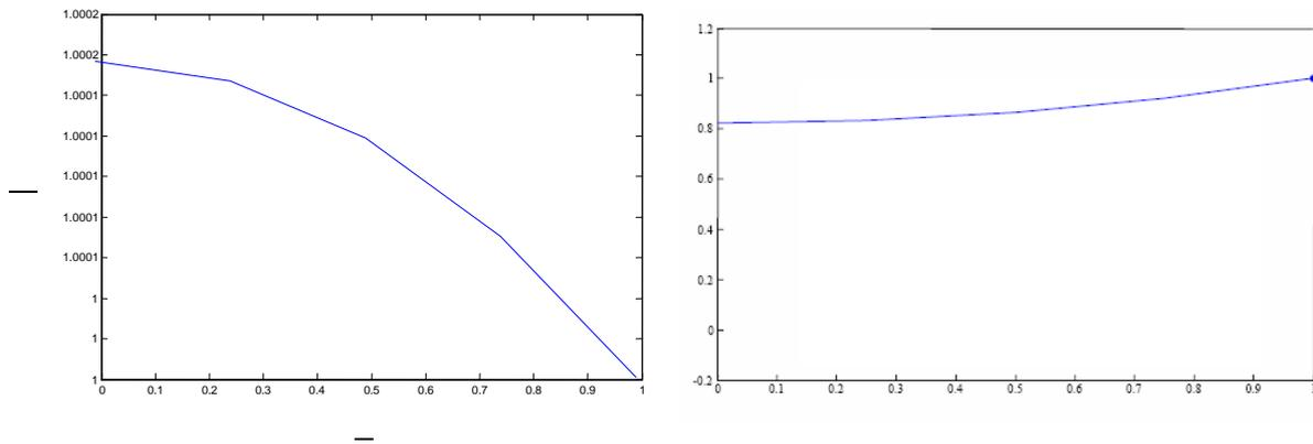
Fig. 1. Temperature profile in catalyst pellet in inlet of the reactor ( :temperature in the catalyst pellet, :catalyst surface temperature)
