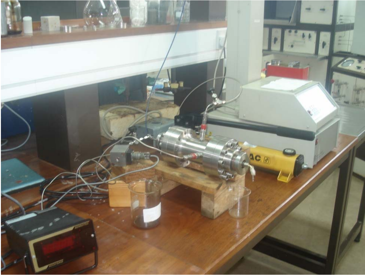
Fig. 1 Experimental setup used in studying geochemical characterization of pH change in core samples
