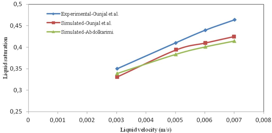
Fig. 7. Comparison of simulated results of mean liquid saturation with data of Gunjal et al.
