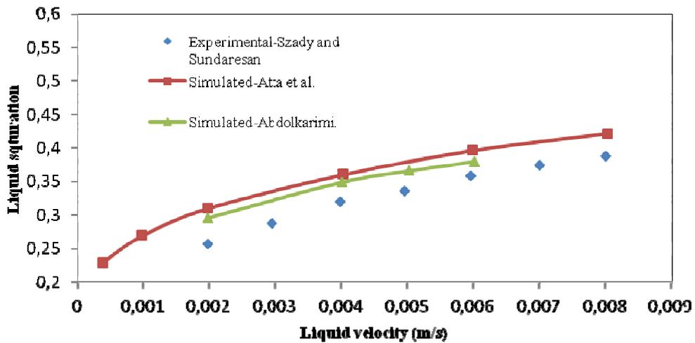
Fig. 5. Comparison of simulated results of mean liquid saturation with data of Szady and sundaresan
