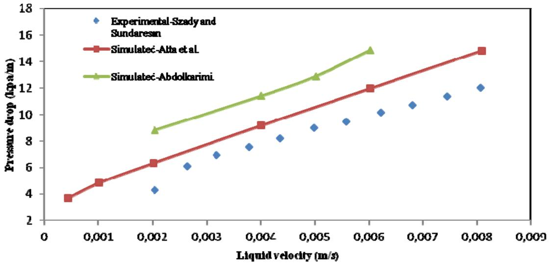
Fig. 4. Comparison of simulated results of pressure drop with data of Szady and sundaresan
