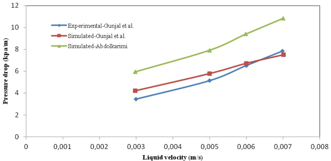
Fig. 6. Comparison of simulated results of pressure drop with data of Gunjal et al.
