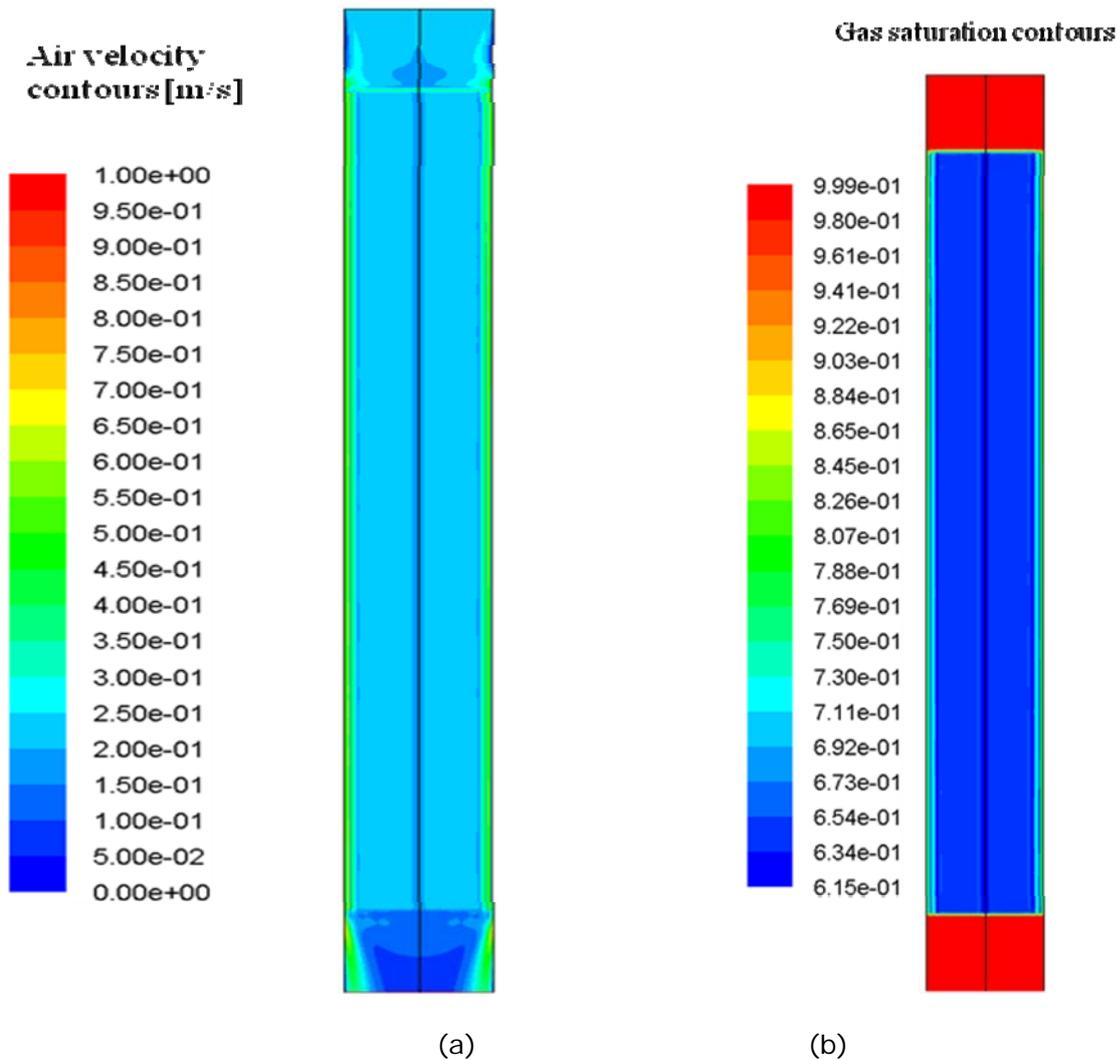
Fig.3 (a)Air velocity contours (b)Air saturation contours through porous media with porosity distribution
