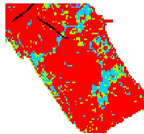
Figure 7 Probability map for a fracture intensity cut-off of 0.5
