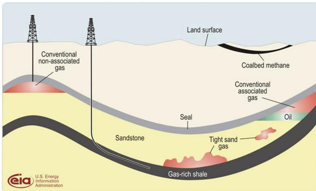
Figure 1. Schematic geology of natural gas resources [23]
