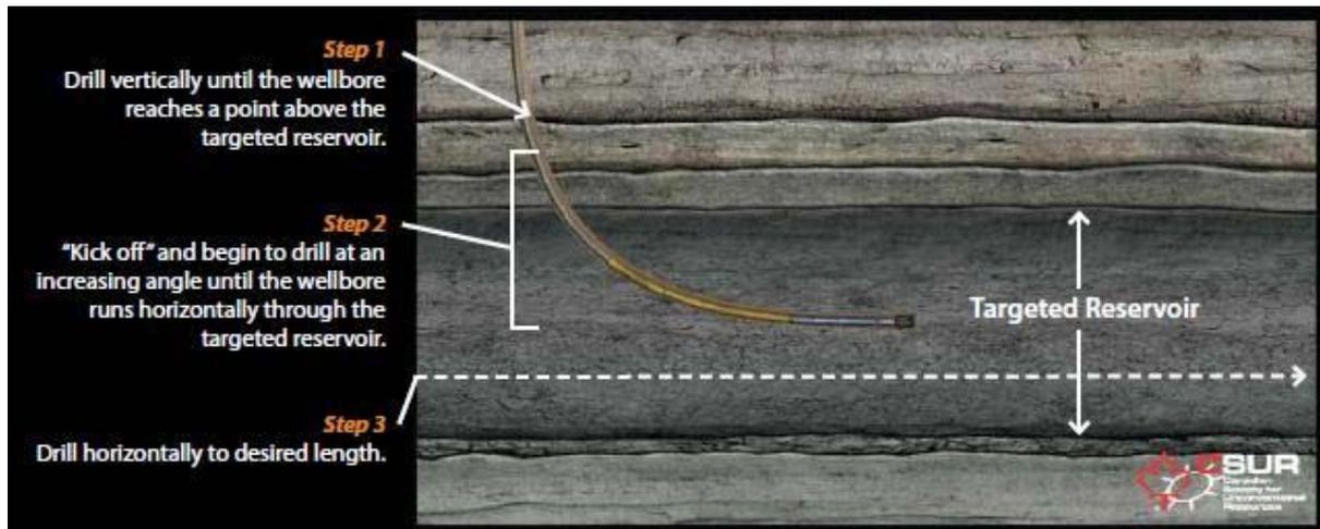
Figure 4. Horizontal drilling [8]
