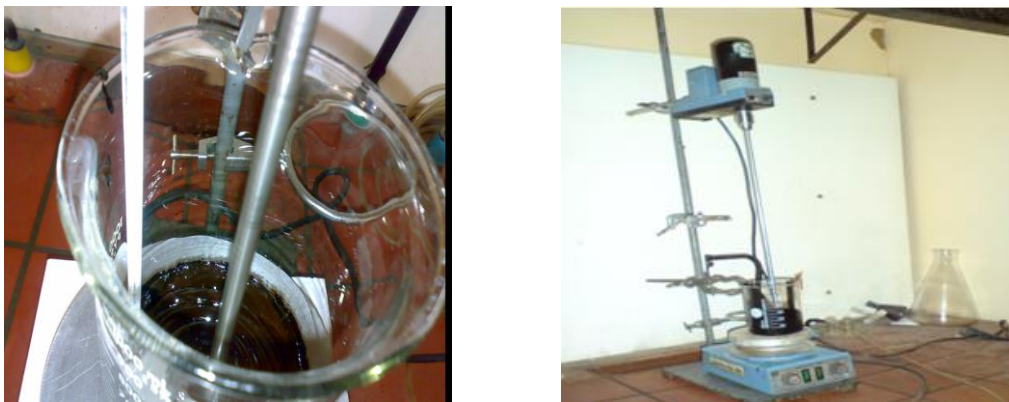
Figure 2 Test run for ODS of fuel oil with chemical on heating & mixing condition
