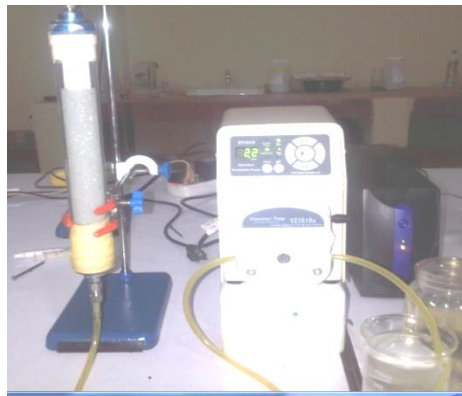
Fig.2 Core saturation with brine.
