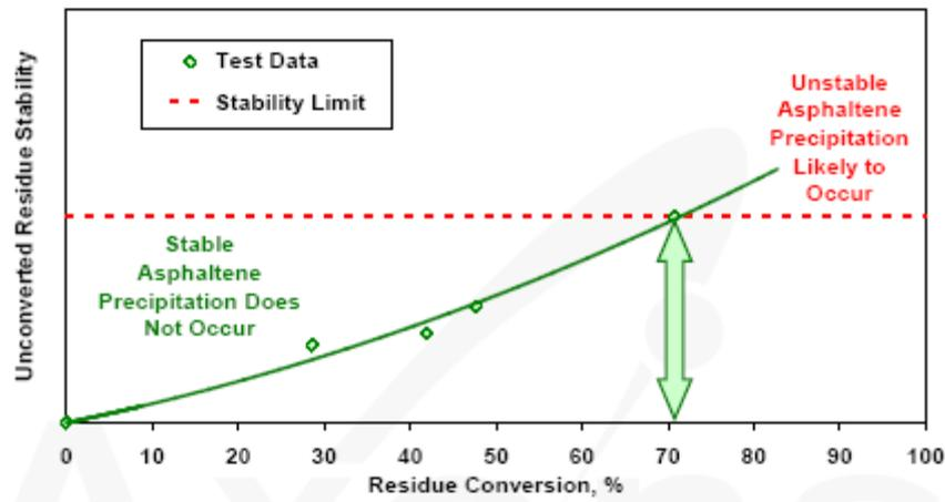
Figure 2 Stability Limit for ebullated bed hydrocracking conversion level [14]
