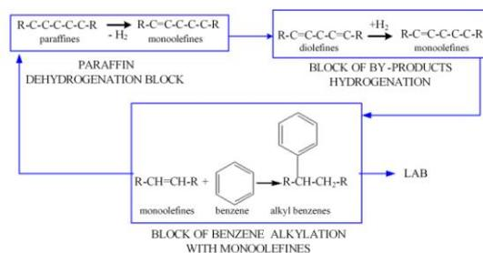
Figure 1. Technological scheme of hydrogenation unit
