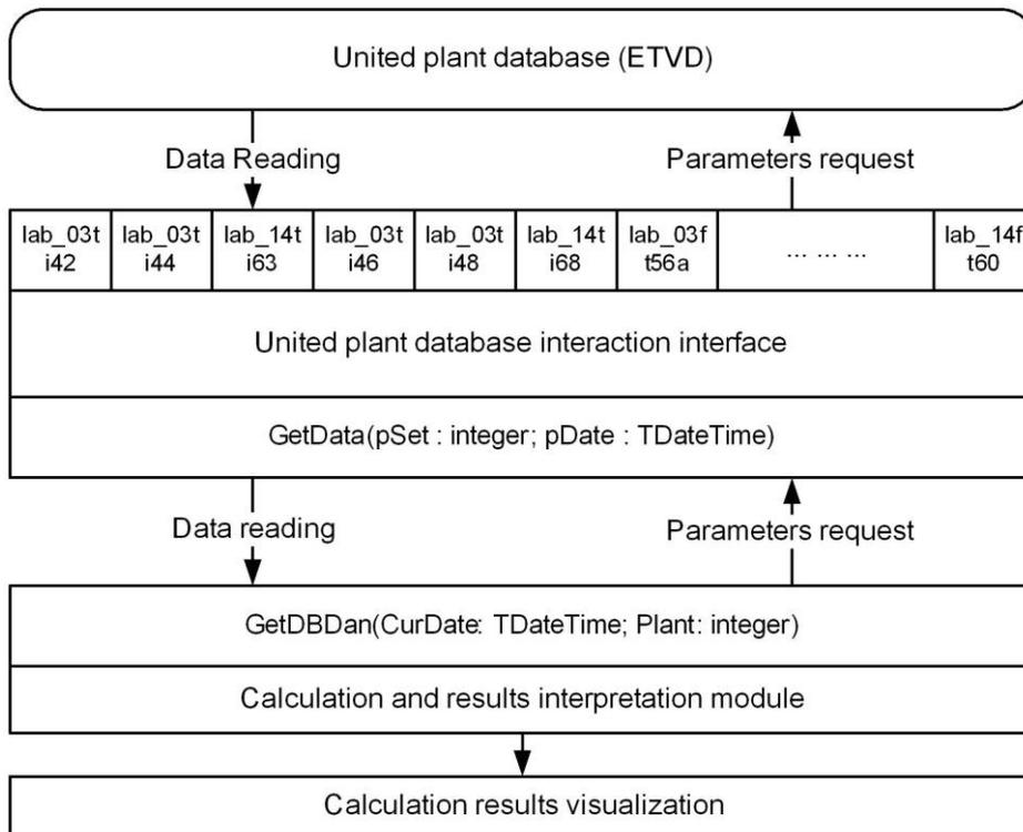
Figure 7. Scheme for connecting module use in modeling program for dienes hydrogenation on nickel-containing catalyst
