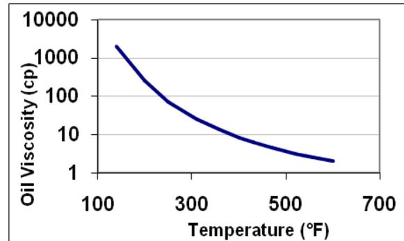
Fig. 2 Oil viscosity versus temperature
