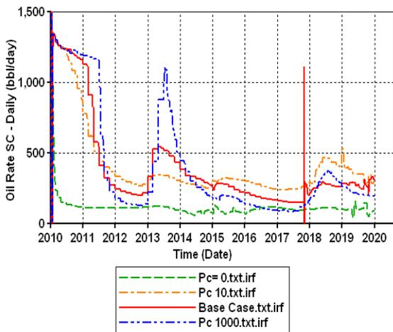
Fig. 8 Effect of matrix capillary pressure on oil production profile in NFR
