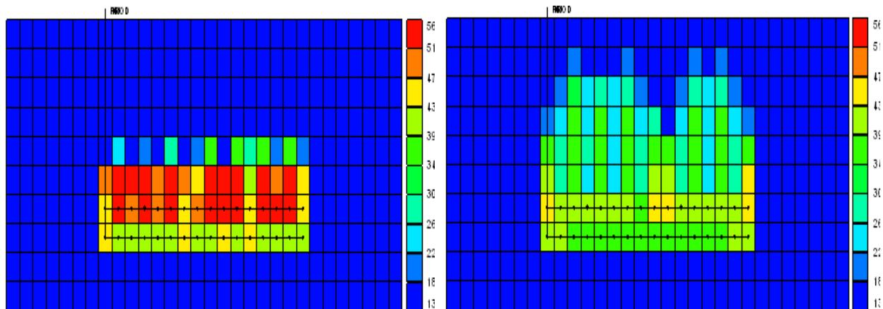
Fig. 7 Temperature profile in base case (left) and oil-wet matrix (right) after 10 years
