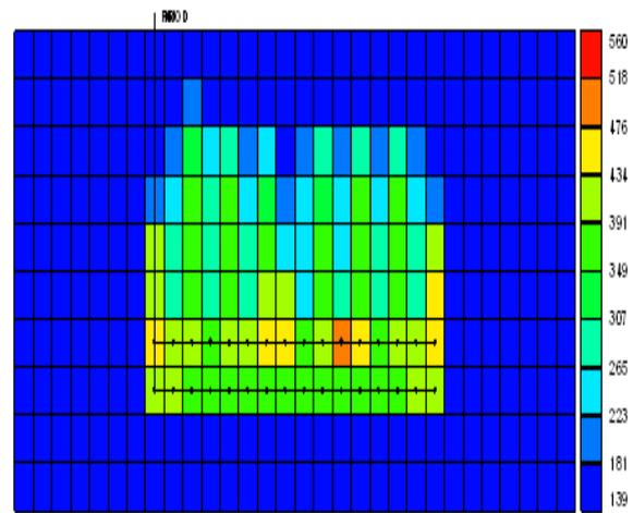
Fig. 9 Temperature profile in case of  $P_c=0$  after 10 years
