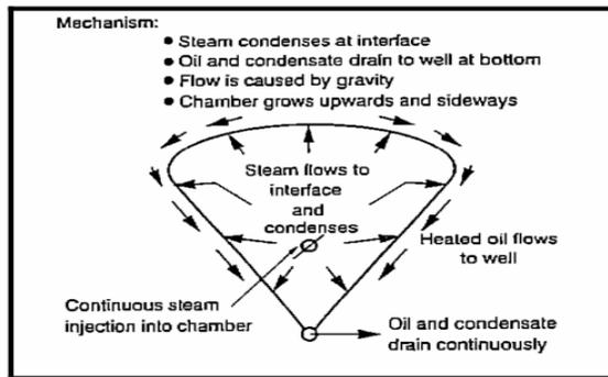
Fig. 1 Essential feature of the SAGD process [1]
