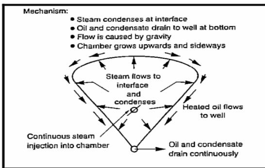
Fig. 1 Essential feature of the SAGD process [1]
