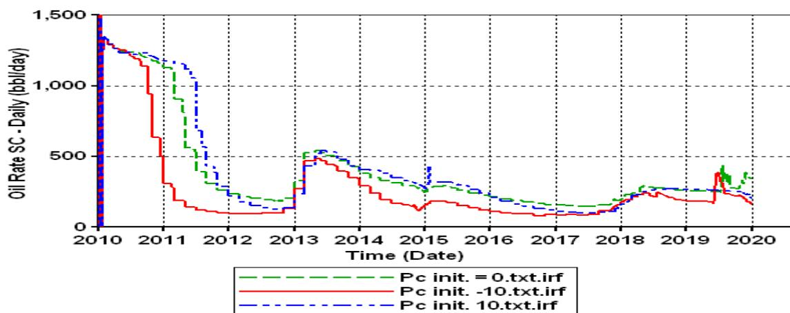
Fig. 10 Effect of threshold pressure on oil production profile in NFR
