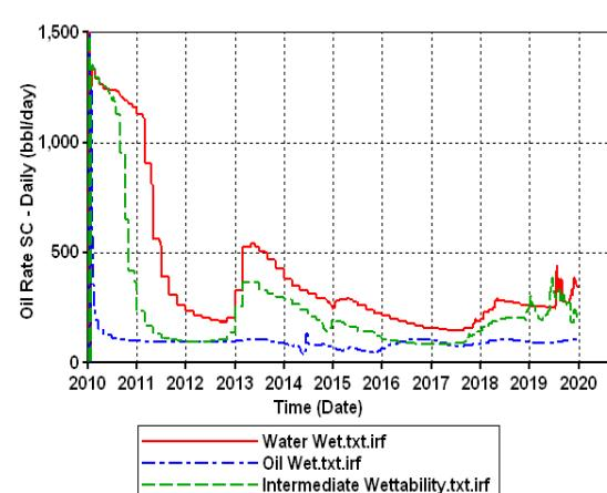
Fig. 6 Effect of matrix wettability on oil production profile in NFR
