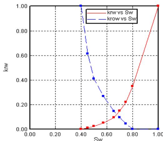
Fig. 3 Oil-water relative permeability
