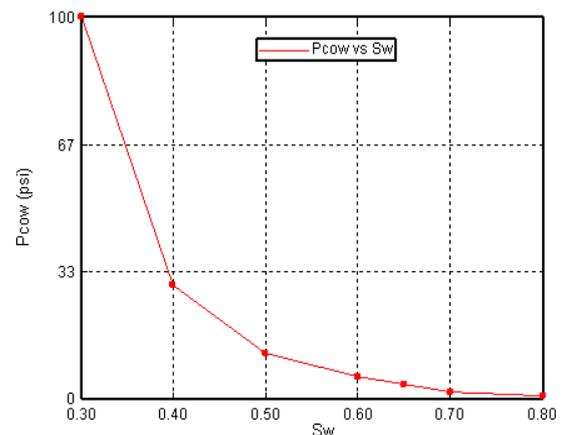
Fig. 4 Matrix capillary pressure curve
