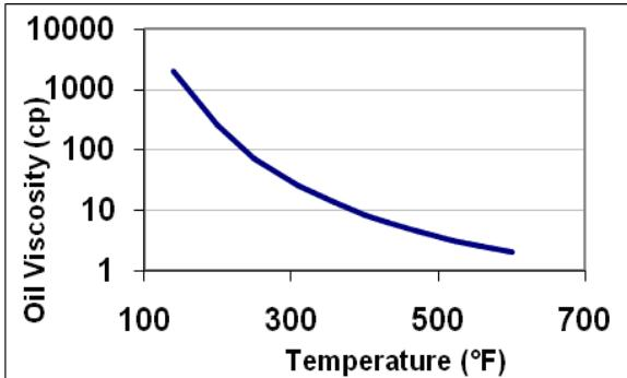
Fig. 2 Oil viscosity versus temperature
