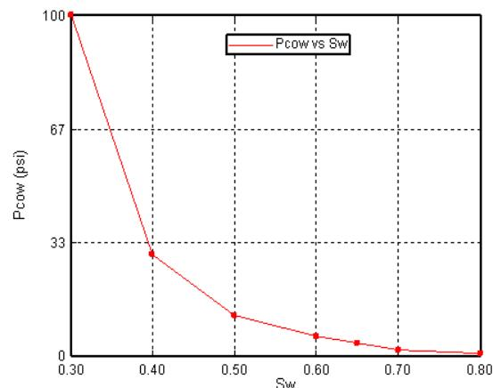
**Fig. 4 Matrix capillary pressure curve**
