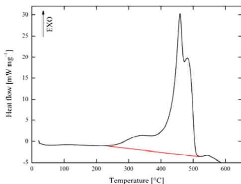
Fig. 1. DSC record of thermooxidative degradation of RHA 4
