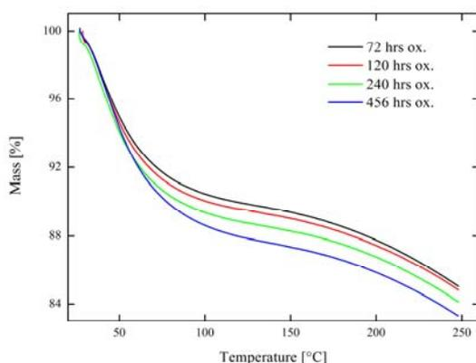
Fig. 5. Evaporation of moisture from samples RHA 4–7
