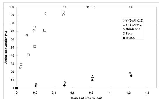
Fig.4. 4-SA conversion versus time related to one gram of the catalysts (150°C, 50 g mixture with the molar ratio aniline/4-SA = 21.5)
