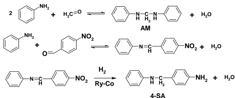
Scheme 2. Synthesis of initial substances, aminal and 4-amino-N-benzylaniline
