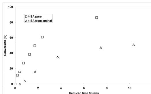
Fig. 6. 4-SA conversion on time related to one gram of the catalyst (150°C, 50 g mixture with the molar ratio aniline/4-SA = 21.5)
