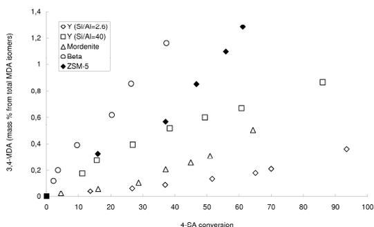
Fig. 1. Formation of 3,4'-MDA isomer from 4-amino-N-benzylaniline over zeolite catalysts (150°C, 50 g mixture with the molar ratio aniline/4-SA = 21.5, 0.3 g zeolite)
