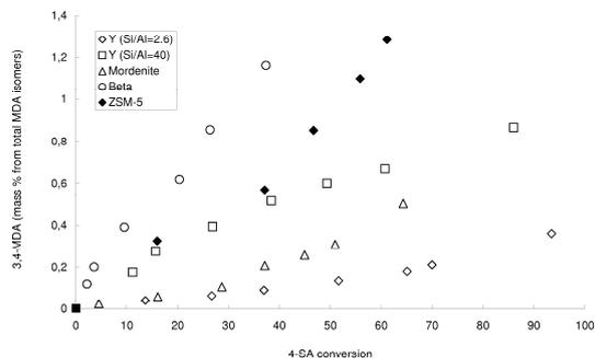
Fig.3. 4-SA isomer content versus aminal conversion (150°C, 50 g mixture with the molar ratio aniline/aminal = 21.5
