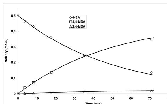
Fig. 8. Comparison of the kinetic model of 4-SA conversion with the experimental data (50 g mixture with the molar ratio aniline/4-SA= 21.5, 0.3 g zeolite Y, Si/Al = 2.6)
