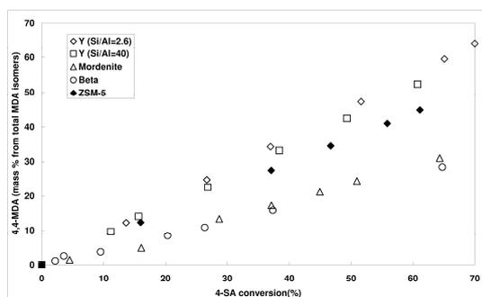
Fig. 5. 4,4'-MDA isomer content versus 4-SA conversion (150°C, 50 g mixture with the molar ratio aniline/4-SA = 21.5
