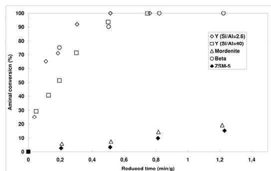
Fig. 2. Aminal conversion versus time relative to one gram of the catalyst (150°C, 50 g mixture with the molar ratio aniline/aminal = 21.5)
