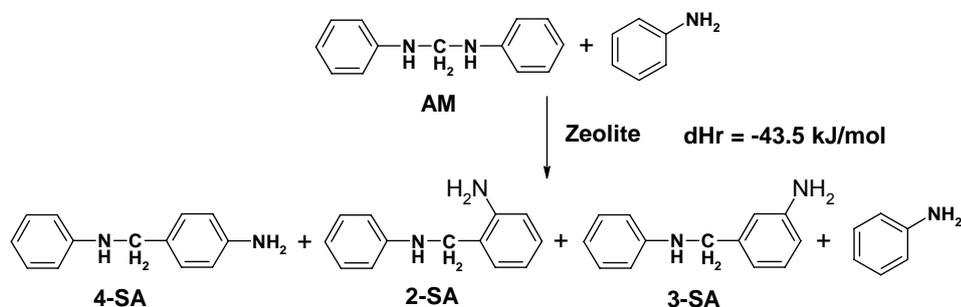
Scheme 3. Synthesis of secondary amines from aminal
