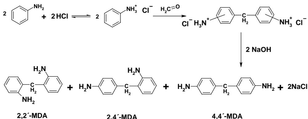
Scheme 1. The traditional procedure of MDA production with the use of HCl as an acid catalyst
