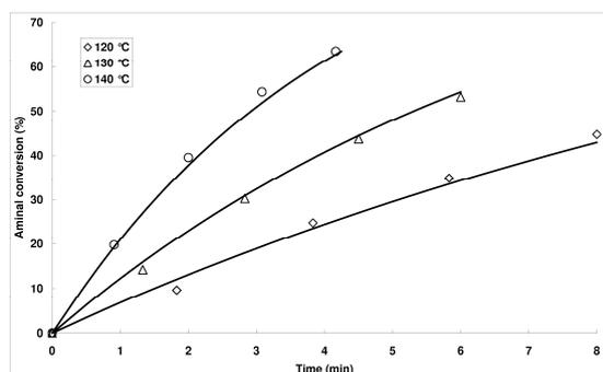
Fig. 7. Comparison of the kinetic model of aminal conversion with the experimental data (50 g mixture with the molar ratio aniline/aminal= 21.5, 0.1 g zeolite Y, Si/Al = 2.6)
