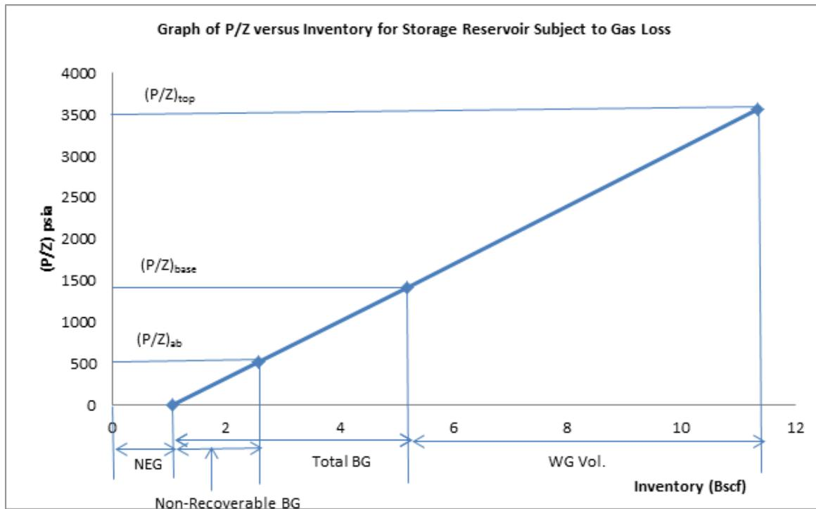
Figure 2 P/Z versus Inventory for storage reservoir subject to gas loss.
