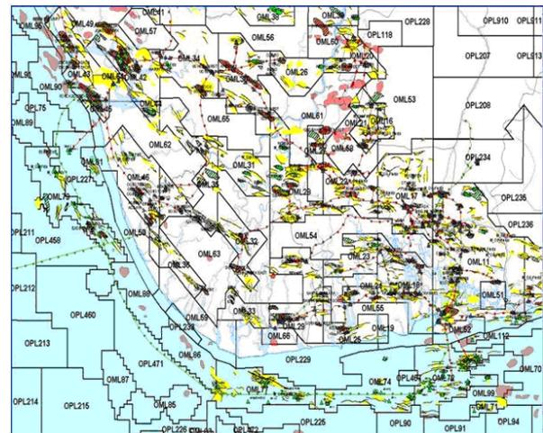
Fig. 2. Prospectivity map of the Niger delta basin showing the different Oil Mining Leases (OML)
