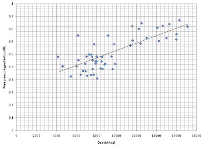
Fig. 11. Pore pressure – depth cross plot showing depth of overpressure occurrence in the study area
