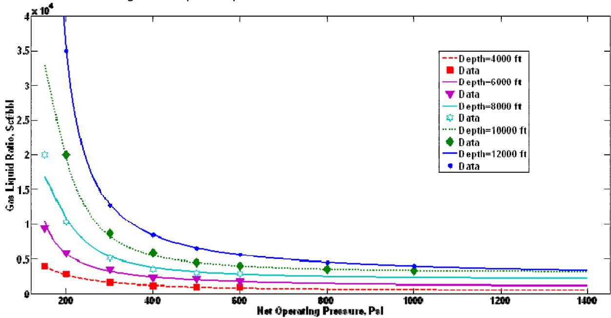
Figure 2. The results of predictive tool for the estimation of minimum gas liquid ration for 2" plunger lift in comparison with Beeson *et al.* [3] data.
