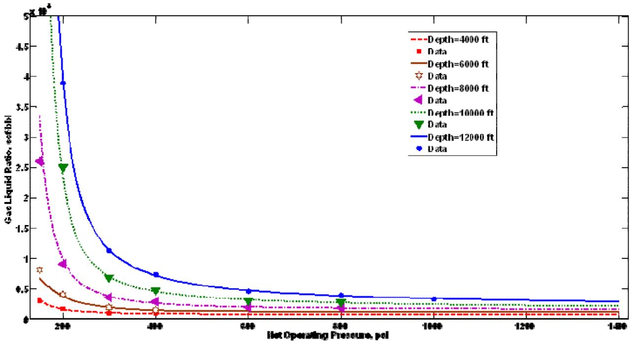
Figure 3. The results of predictive tool for the estimation of minimum gas liquid ration for 2.5" plunger lift in comparison with Beeson *et al.* [3] data.
