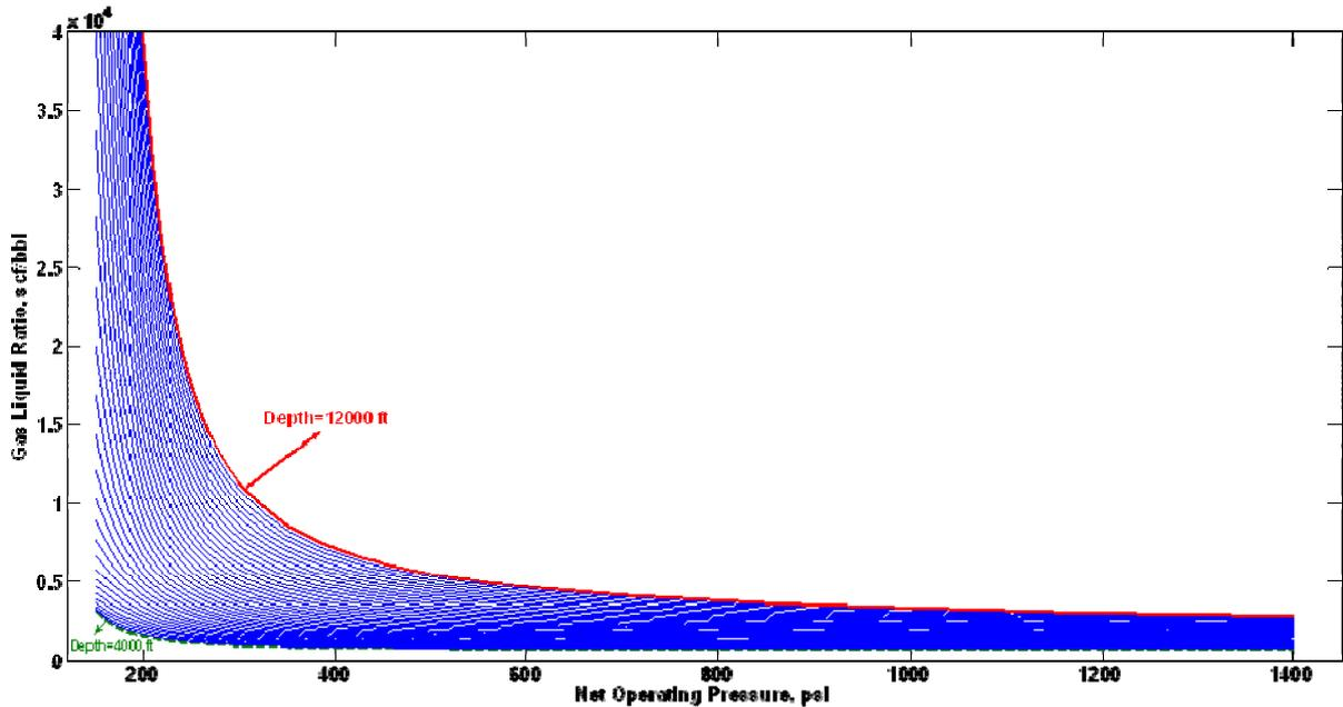
Figure 5. The performance of predictive tool for the estimation of minimum gas liquid ration for 2.5" plunger lift
