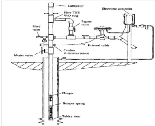
Figure 1. Installation of Plunger lift in a well
