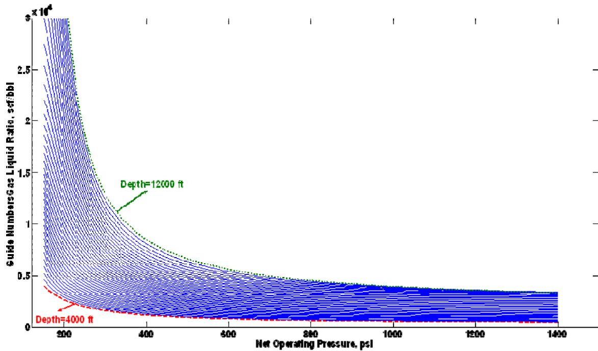
Figure 4. The performance of predictive tool for the estimation of minimum gas liquid ration for 2" plunger lift.
