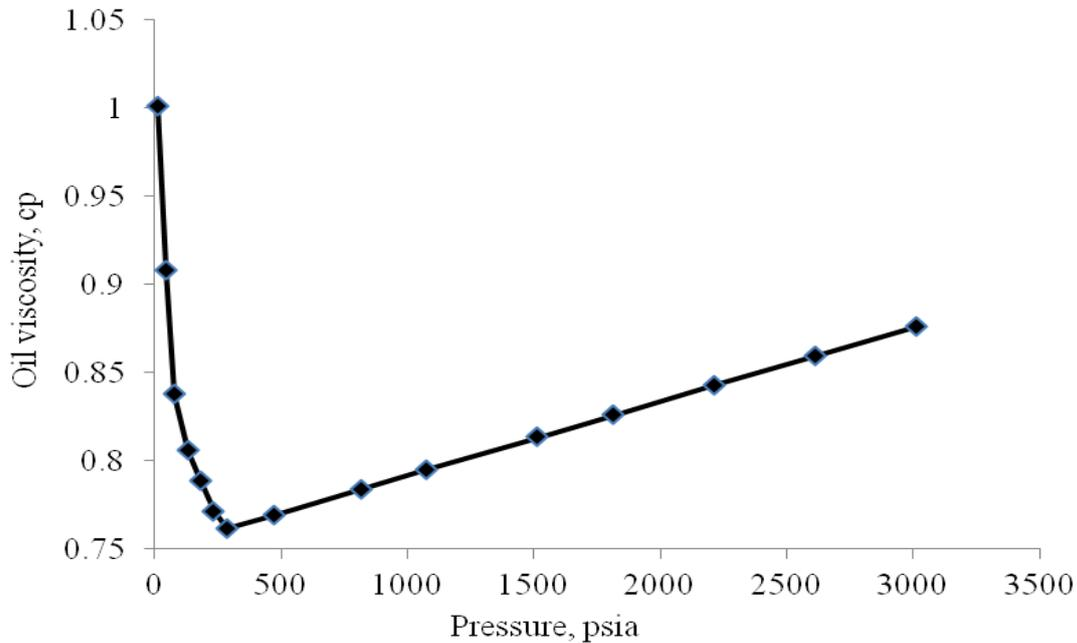
Figure 1 Oil viscosity as a function of pressure
