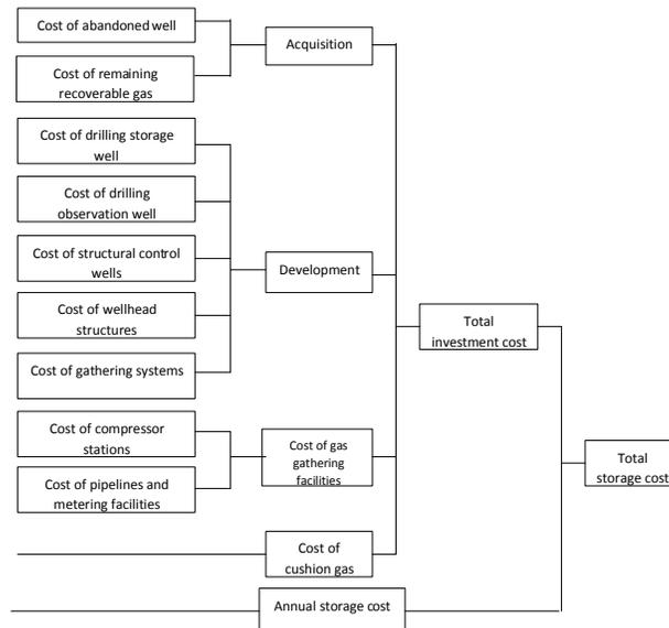
Fig 2.1 Economic flow chart for natural gas storage in depleted reservoir
