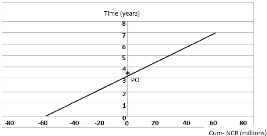
Fig 3.4 Plot of Time in Years Against Cum-NCR in Millions of Dollars, Reservoir Z-16T
