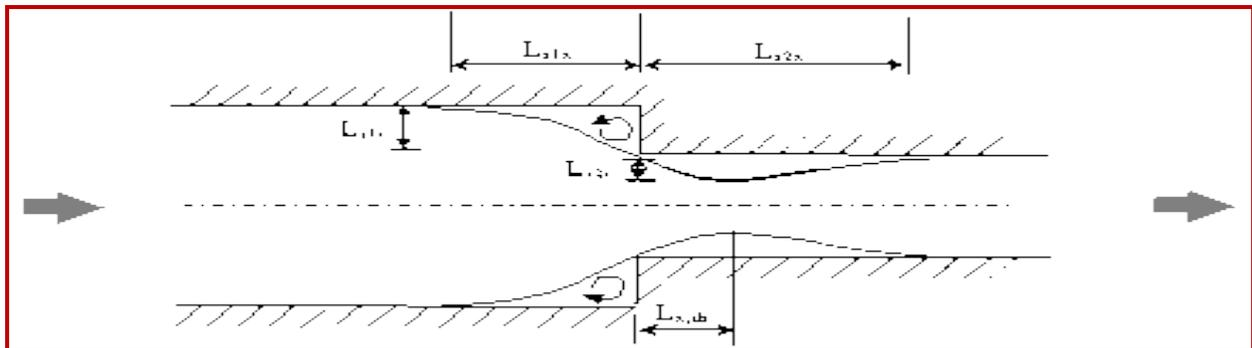
Figure 2. The upstream and downstream separations in the vicinity of the contraction
