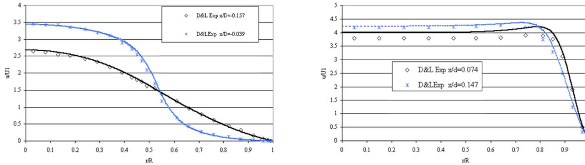
Figure 5 Comparison of predictions and experimental results at Re=196
