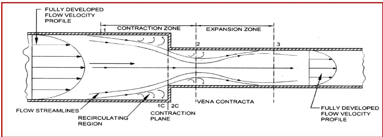
Figure 1. The flow through a sudden pipe contraction
