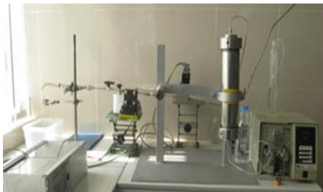
Figure 1 Foam preparation with specific quality system in surrounding pressure and temperature
