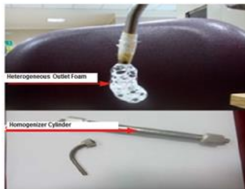
Fig. 3 The obtaining foam before connecting homogenizing factor and homogenizing cylinder that is shown at the figure
