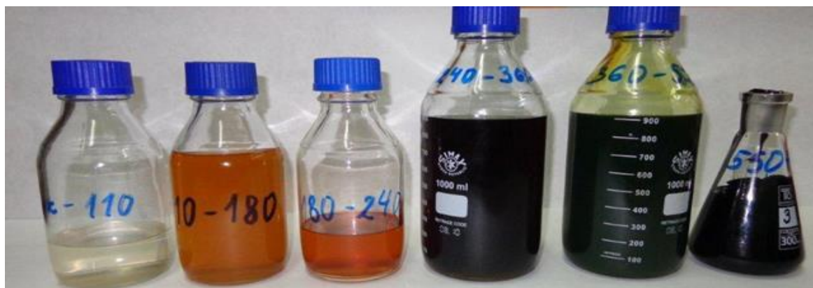
Fig. 4. Photograph of appearance of the wide fractions obtained during TBP distillation of the blend 20% waste tyre pyrolytic oil / 80% REBCO
