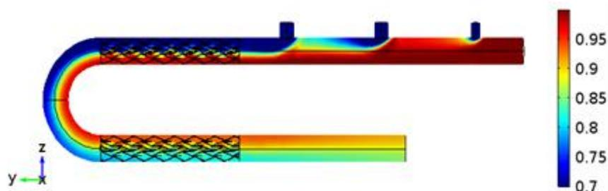
Figure 3. Volume fraction of ethylene at second option (t = 2 sec)
