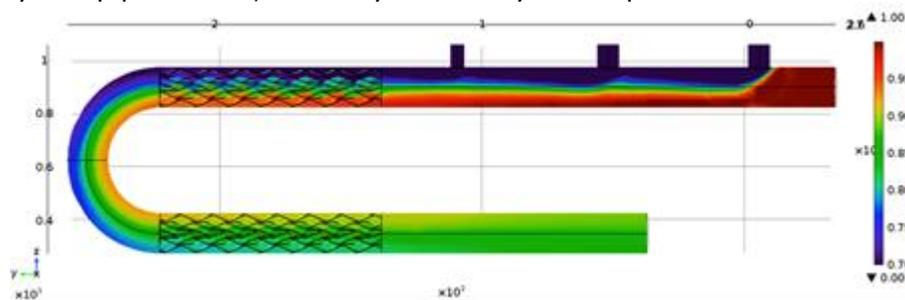
Figure 4. Volume fraction of ethylene at third option (t = 2 sec)
