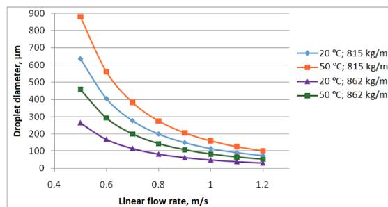
Fig. 3. Dependence of the droplet diameter on the linear flow rate, temperature, and oil density
