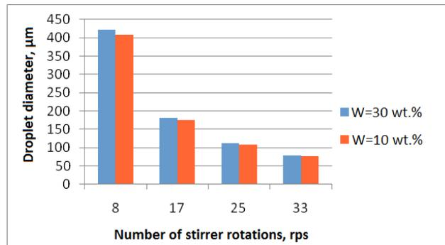
Fig. 1. Dependence of the average droplet diameter on the number of the stirrer rotations (the temperature is equal to 20°C; the oil density is equal to 815 kg/m<sup>3</sup>)
