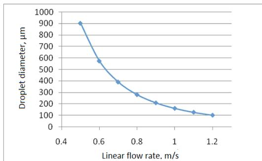
Fig. 2. Dependence of the droplet diameter on the linear flow rate (the temperature is 50°C; the water content is 10 wt.%; the oil density is 815 kg/m<sup>3</sup>)
