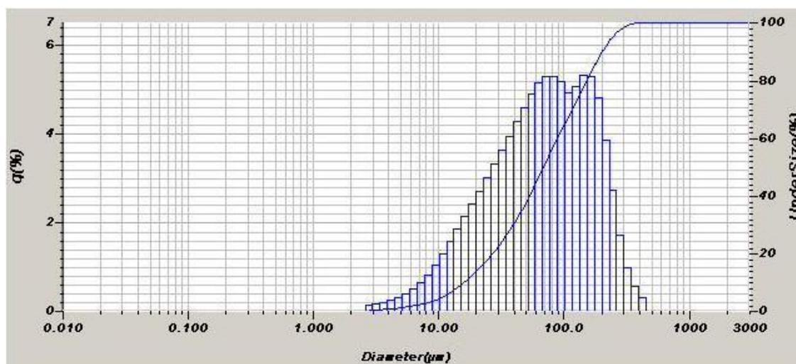
Figure 2. The catalyst particles distribution by diameter
