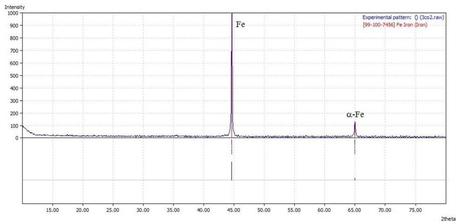
Figure 5. The catalyst derived in media of carbon dioxide radiograph
