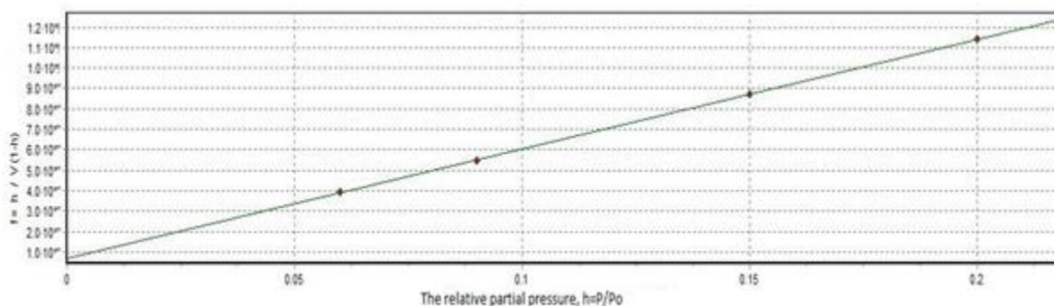
Figure 3. BET adsorption isotherm
