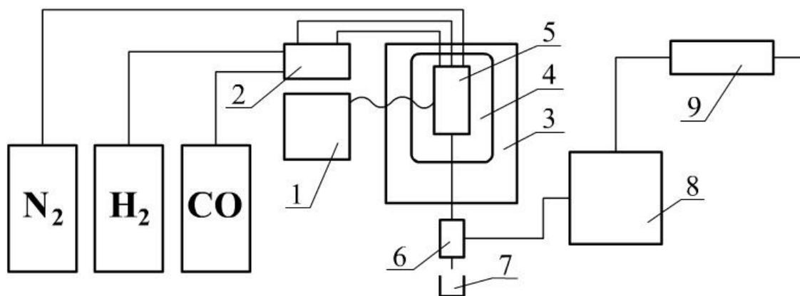
Figure 1. Catalytic unit scheme: 1 – temperature controller, 2 – gas metering unit, 3 – heat chamber, 4 – reactor jacket, 5 – reactor, 6 – separator, 7 – receiver, 8 – gas chromatograph, 9 – air vent.
