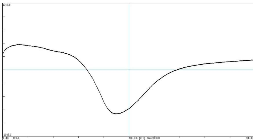
Figure 7. Iron powder electro-paramagnetic resonance spectrum
